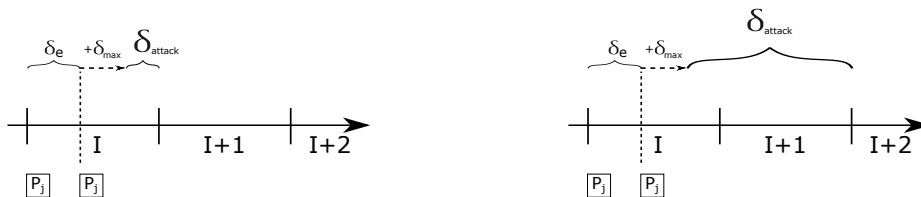
Fig. 6. Illustration of the difference between the original TESLA (right) security condition, and the slightly changed version of ASTS (left).
