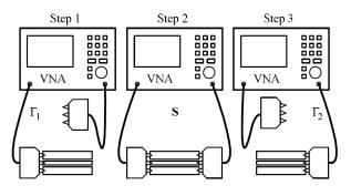
Fig. 2. Verification measurement steps.
