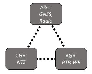
Fig. 1. The Time Transfer Trade-off Triangle, where A signifies "accurate", C signifies "convenient", and R signifies "reliable".
