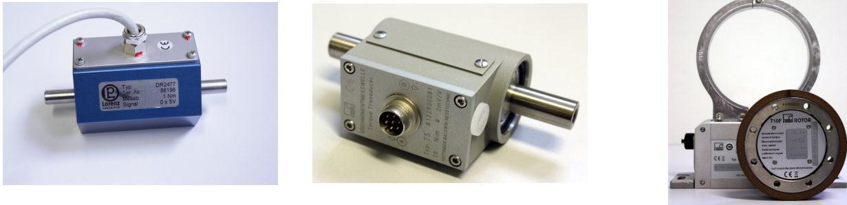
Figure 5: Analysed torque transducers, 1 N · m shaft type (left), 10 N · m shaft type (middle), and 50 N · m flange type (right).
