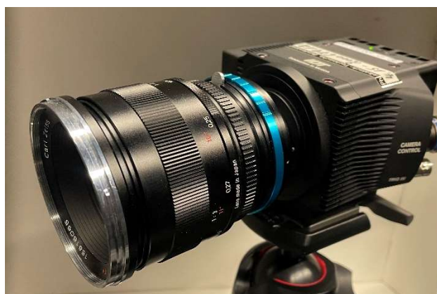
Figure 1 – Photo of the high-speed camera IDT OS 7 - S3 from Imaging Solutions GmbH with a ZF.2 Makro-Planar 2/50 lens from Carl Zeiss.
