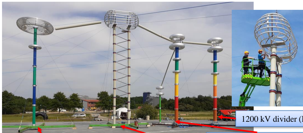
2000 kV divider (PTB)
