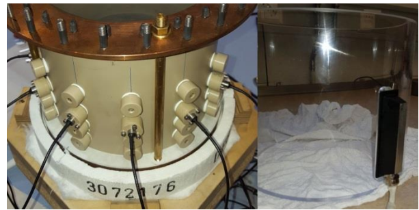
Figure 2: View to the instrumentation for the flow measurements. On the left side the option with single transducers and on the right with the ultrasound array. The single transducers are coupled through holes directly to the melt whereas the UDV array measures through the wall of 2.3 mm thickness.
