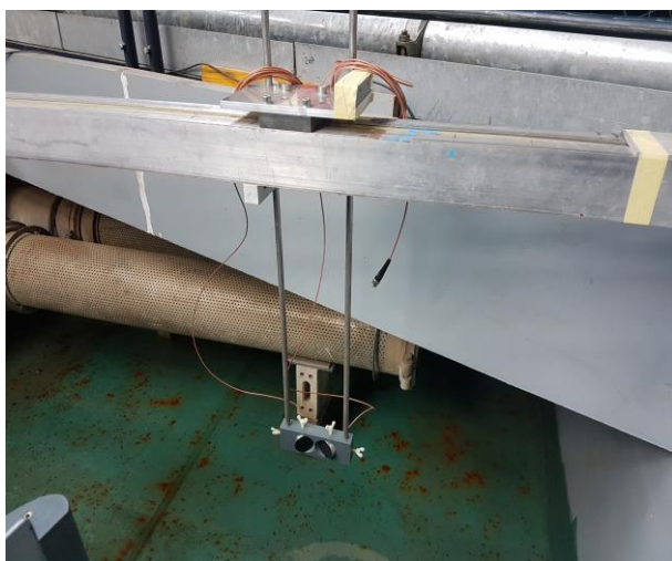
Figure 3 UVP sensors, frame and carriage
