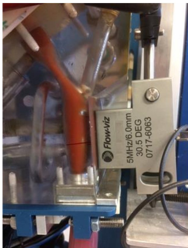
Figure 2: Photo of the customized UVP sensor measuring the flow of ketchup inside the pharynx.
