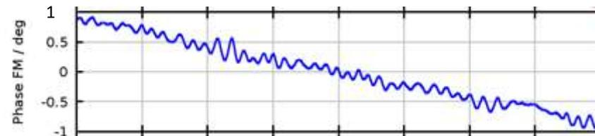
4 WT, in 8 km distance to DVOR, 140 m hub height, 112 m rotor diameter
