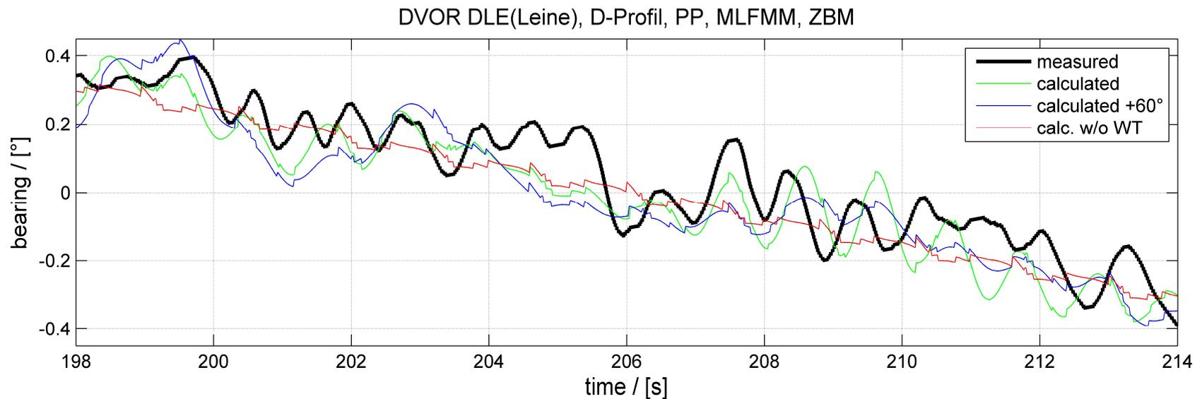
Horizontal flight track 100 m behind WT in 2.5 km distance to DVOR:
