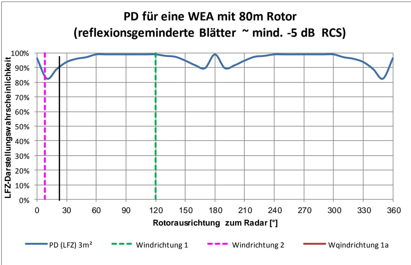
Rotoraxis is orientated to the radar
