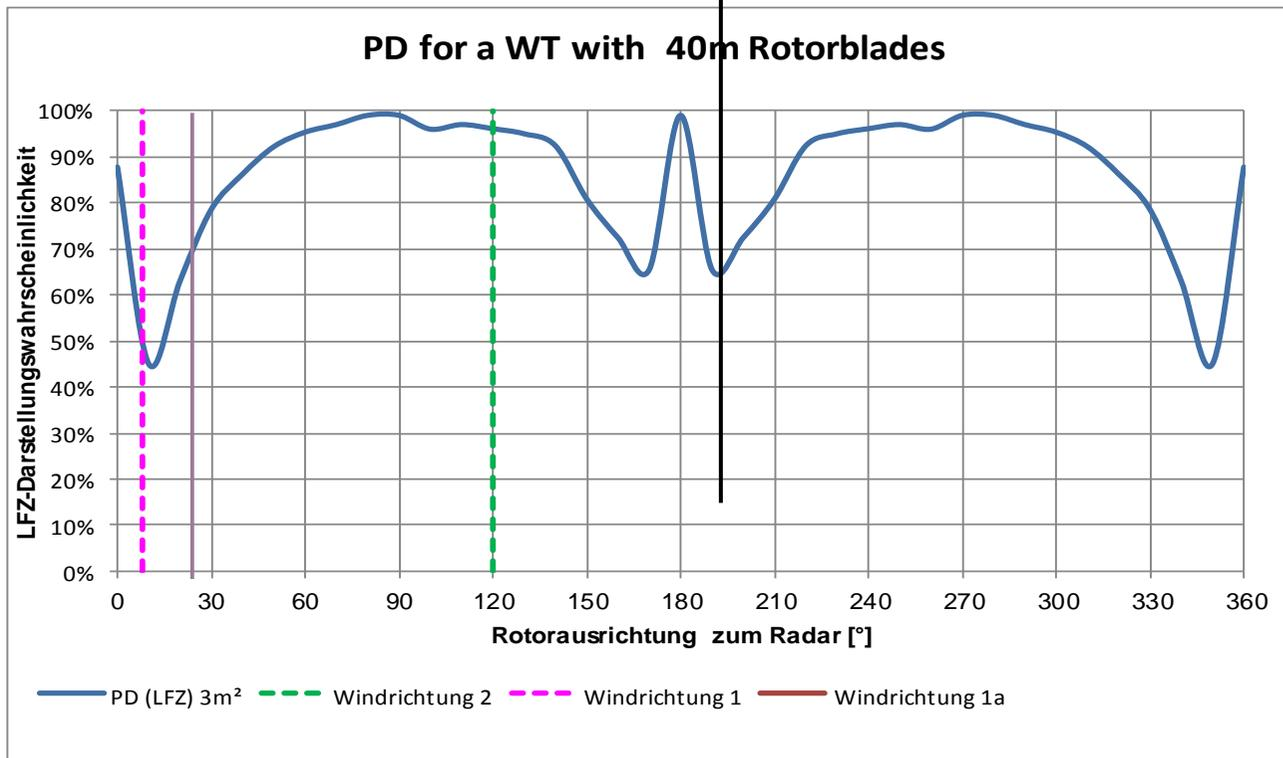
At 180° : Rotoraxis is orientated to the radar (here we don't have an aircraft loss)
