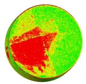
Figure 6: Colour-coded representation of the LQV for a CT-scan of a cylinder (aluminium; height 12 mm, diameter 18 mm) with several layers of adhesive tape attached. The LQV is assessed by evaluating the homogeneity of the grey values along the surface and the sharpness of the transition from low to high grey values on a line perpendicular to the surface
