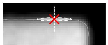
Figure 3: Zoom of a cross section of the volume data. The red 'x' marks an extracted surface point. The grey values are extracted from a line perpendicular to the surface and an area along the surface, marked in white.
