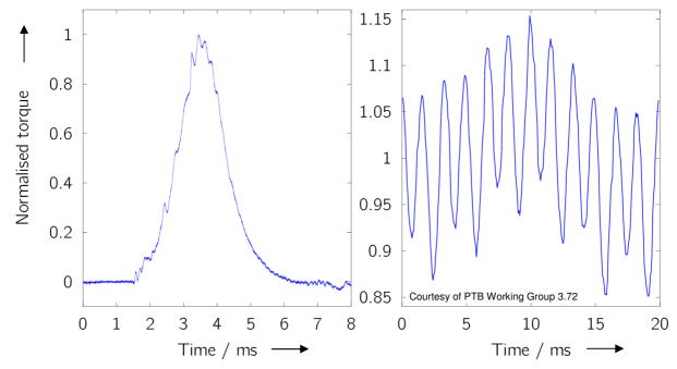
Figure 1a: Fastening cycle of an impulse wrench (left).
