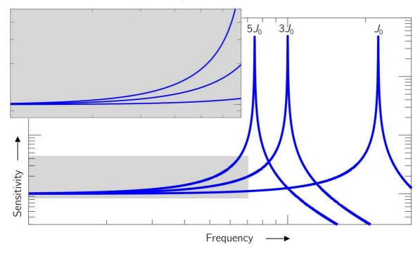
Figure 2: Frequency response of a transducer modelled as a SDOF system with different coupled MMOI resulting in a change of the frequency-dependent sensitivity.
