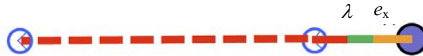
Figure 11. External measurement during birdbath calibration. Measurement of the distance between the SMR locations is unaffected by e_x and \lambda as they are common to both measurements and therefore cancel.
