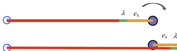
Figure 13. Two-face measurements separate correlated error parameters. In front-face mode (upper), the target range is in error by the sum of e_x and \lambda , whereas in rear-face mode (lower) the sign of e_x has been reversed.
