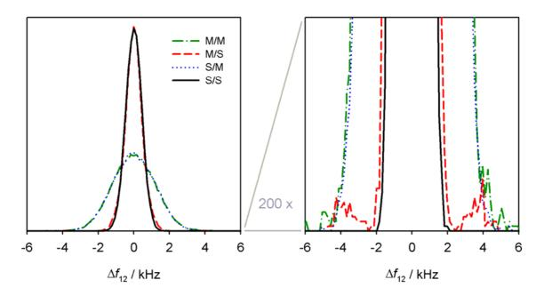
Figure 4: Histograms for 1 second samples of  $\Delta f_{12}$  when the repetition frequency is measured (M) or servo controlled (S). First comb is CMI Ti:Sa, second BEV fibre, respectively. In the right hand side of the picture the ordinate is enlarged by 200 times to demonstrate small differences in the side wings.
