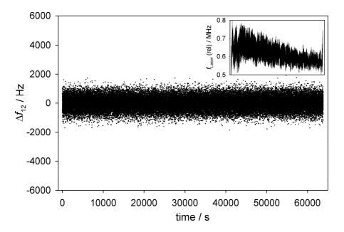
*Figure 2: Deviations of individual 1 s samples between the two combs CMI Ti:Sa and BEV fibre. The inset shows the actual laser frequency relative to an offset 473 612 521 MHz.*
