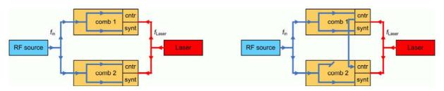
Figure 1: Schematic setup for a comb-comb comparison. Left setup without synchronisation, right with counter synchronisation. cntr: counter, synt: RF-synthesizer. RF signals are denoted by blue lines and  $f_{in}$ , optical signals by red lines and  $f_{Laser}$ .
