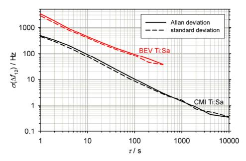
*Figure 3: Allan standard deviation (solid lines) and sample standard deviation (dashed lines) for the frequency difference between BEV fibre comb and the two other combs considered.*
