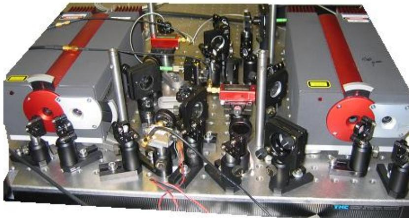
Figure 2 : SW generation system (breadboard 1 – dimensions: 0.45m x 0.60m)
