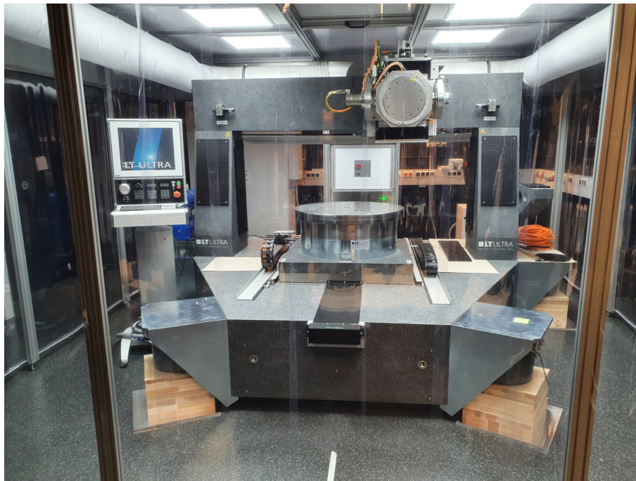
Figure 8.16: Positioning system of the form measurement system for large specimens at PTB.
