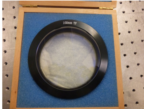
Figure 6.1: Image of the specimen: The transmission flat of a 4 inch Fizeau interferometer.
