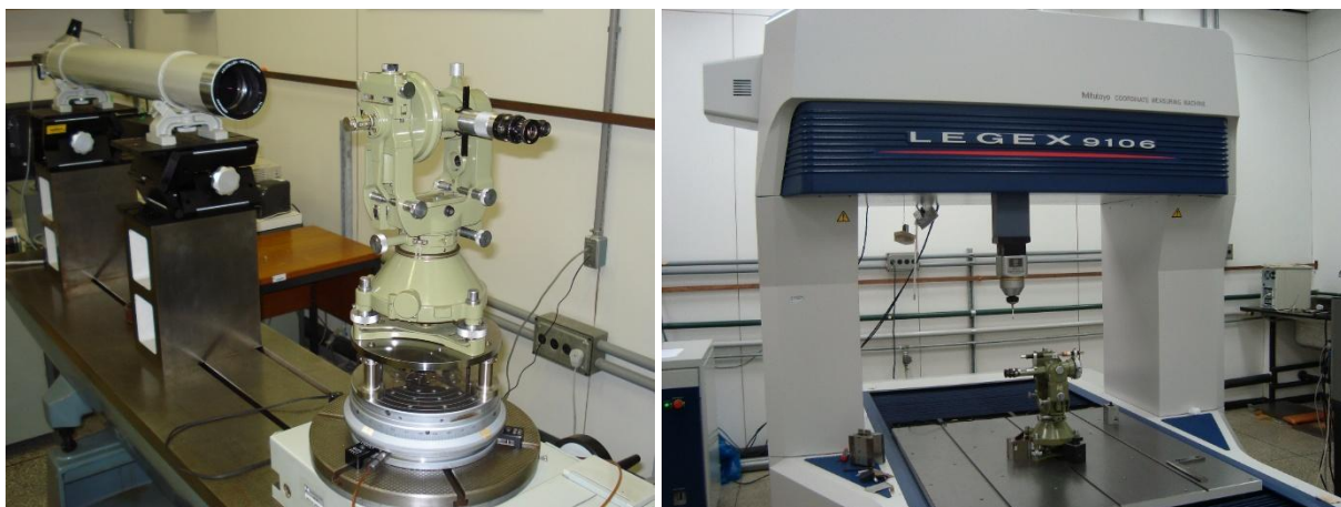
Figure 1: Experimental approach: on the left, the system for calibration of the horizontal scale of theodolites and total stations; on the right, the coordinate measuring machine adopted to support the design of experiments [12].
