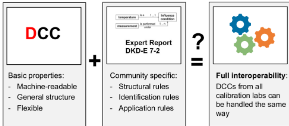
Figure 1. Assumption of full interoperability when adhering to the DCC schema and community specific rules
