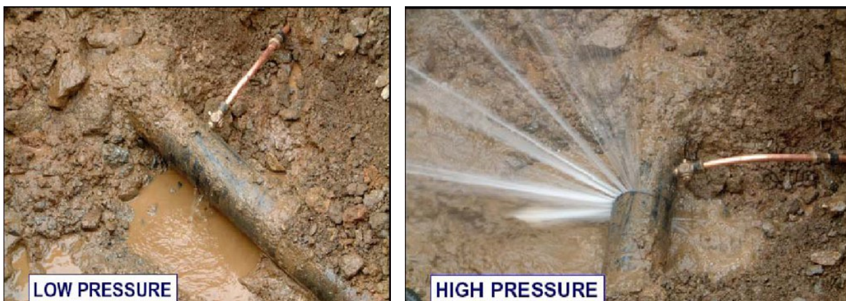
Figures 3.3: Typical leakages left with low pressure and right at high pressure condition, photos provided by Miyahuna (M. Abualshaikh), 2023.
