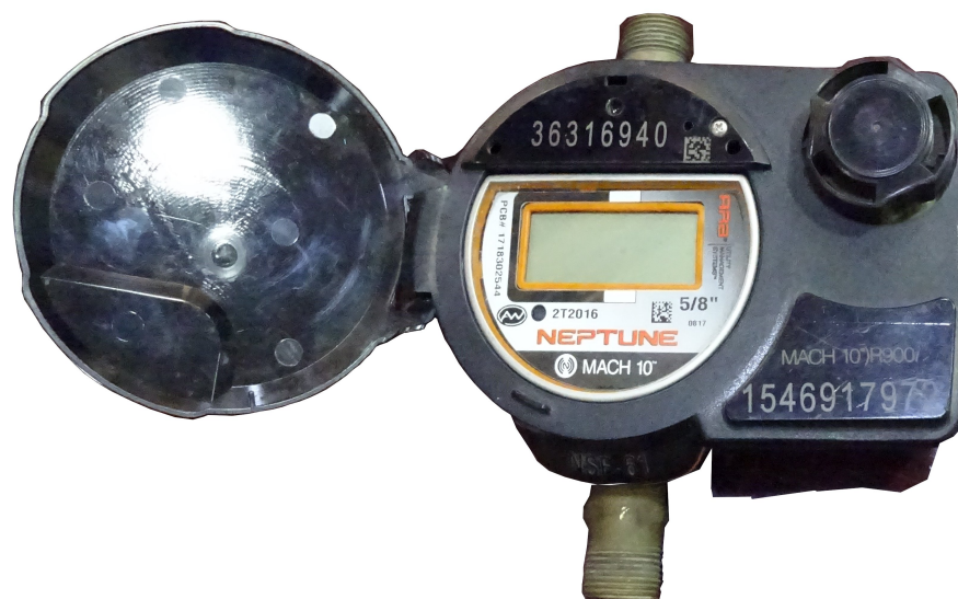
Figure 2.2 Ultrasonic meter with opened lid, produced by Neptune, image by J. Steinbock, Aqaba (2022).
