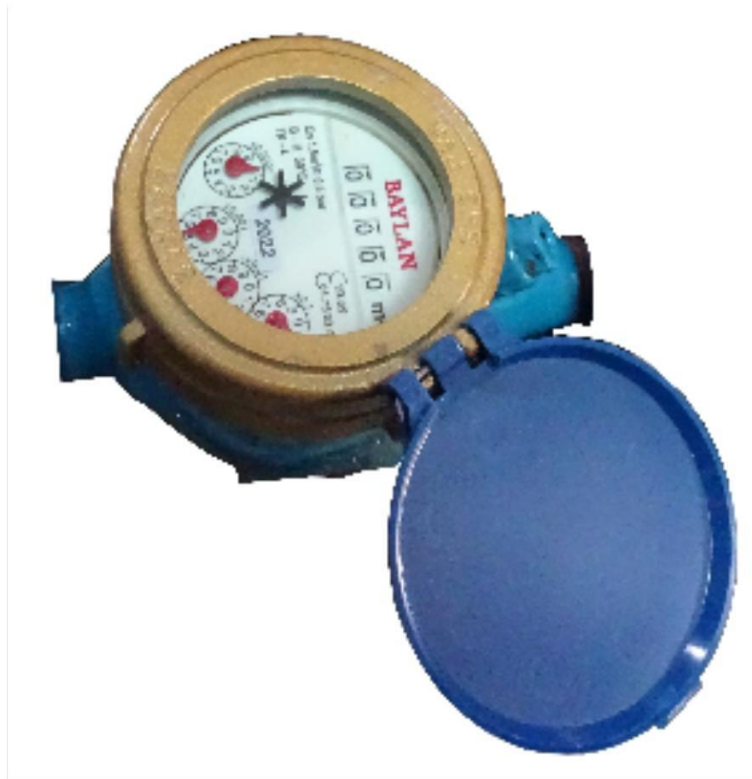
Figure 2.1 Typical mechanical meter with opened lid, produced by Baylan meters, refurbished by WAJ, image by J. Steinbock, Amman (2022).
