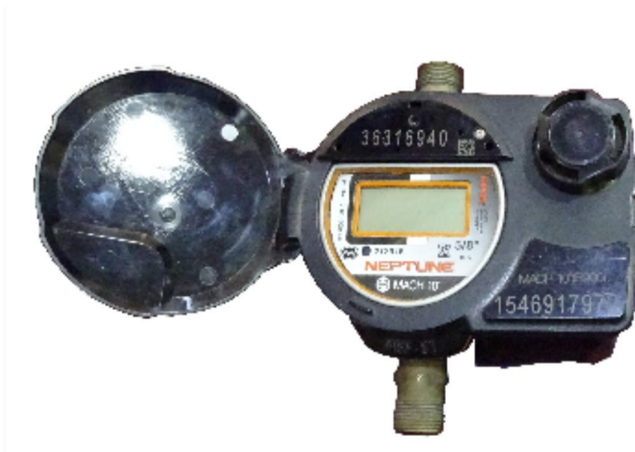
Figure 2.2 Ultrasonic meter with opened lid, produced by Neptune, image by J. Steinbock, Aqaba (2022).
