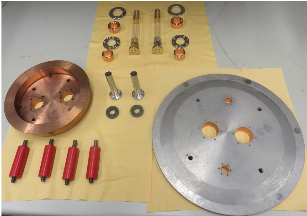
Figure 4.10: Mechanical components of waveguide microcalorimeter.
