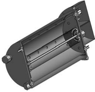
Figure 1: CAD drawing, showing a cut through the pulse ionization chamber. The length of the electrodes is 370 mm and the inner diameter of the outer electrode is 168 mm.
