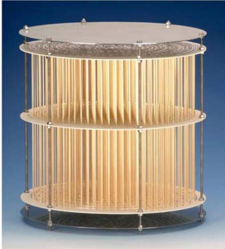
Figure 3: Multi-wire-puls-ionization-chamber for large volume radon detectors, designed by PTB [12]. The sensitive volume of the VIIC marked with (2) in Figure 2 is displayed here. The gold plated wires are connected to different electrical potential, to separate and collect the ions formed by \alpha -particles passing through the air. The electrodes are distributed over a diameter of about 250 mm and have a length of 300 mm.
