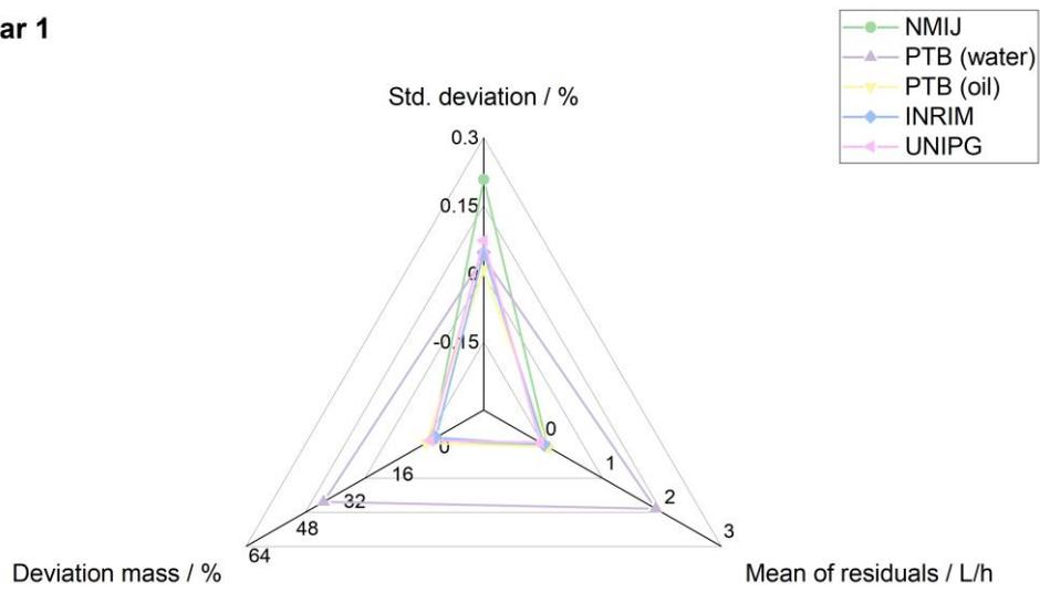
Figure 12: Comparison of the generation of the passenger car profile 1 based on the mean value of the residuals, the deviation of the mass from the specification and the repeatability.
