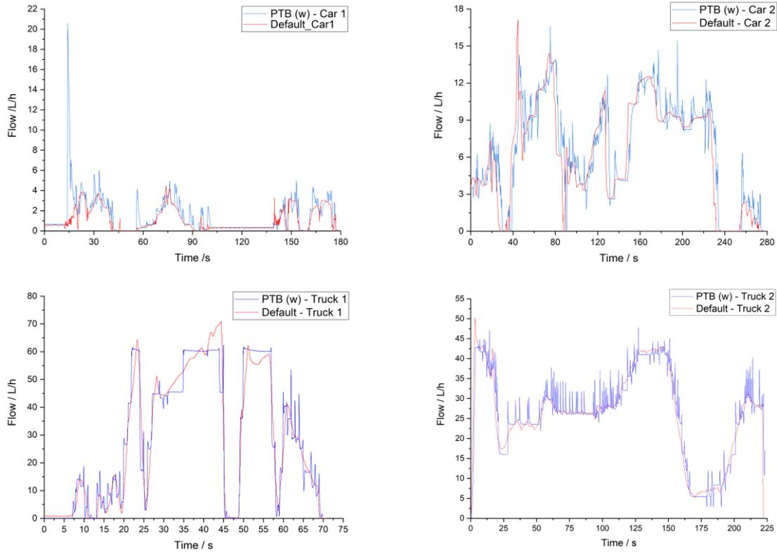
Figure 7: Profile realization PTB water.
