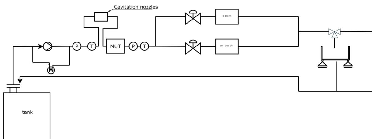
Figure 18: Principal setup of the test bench for measurements using dynamic flow rates at PTB (oil).
