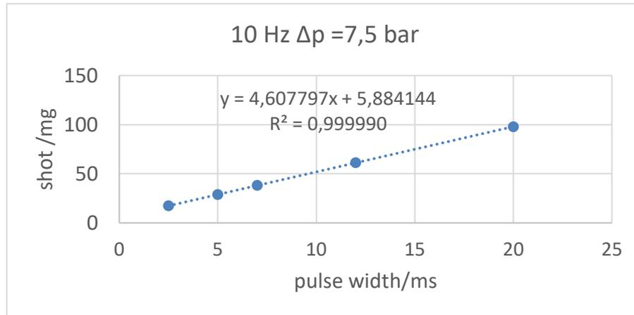
Figure 20: Calibration example.
