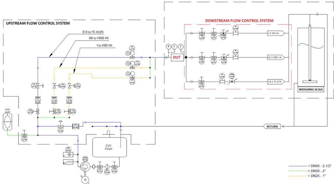
Figure 16: Schematic of Cetiats dynamic test bench.
