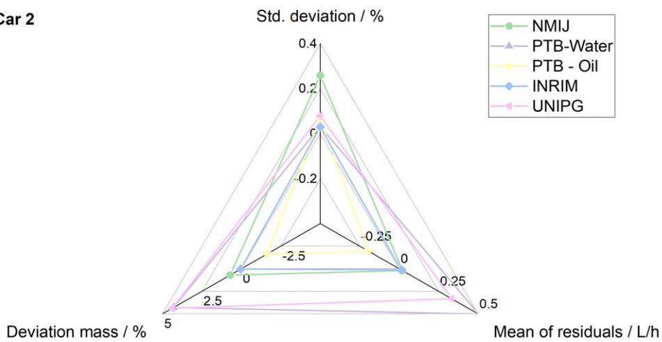
Figure 13: Comparison of the generation of the passenger car profile 2 based on the mean value of the residuals, the deviation of the mass from the specification and the repeatability.
