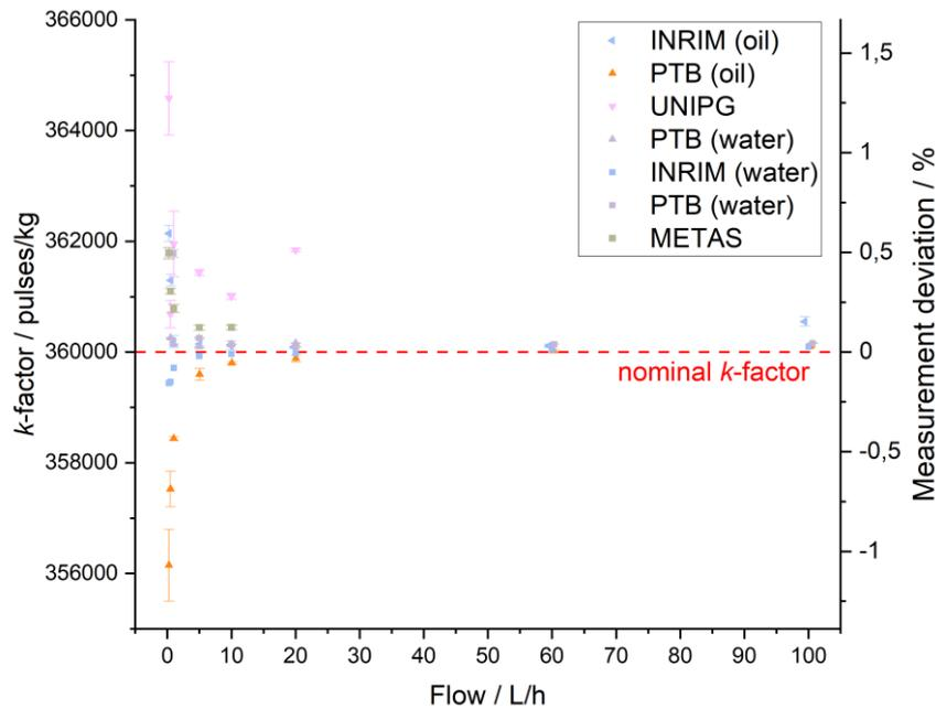
Figure 4: Results of the static measurements (■ water, ▲ calibration oil).
