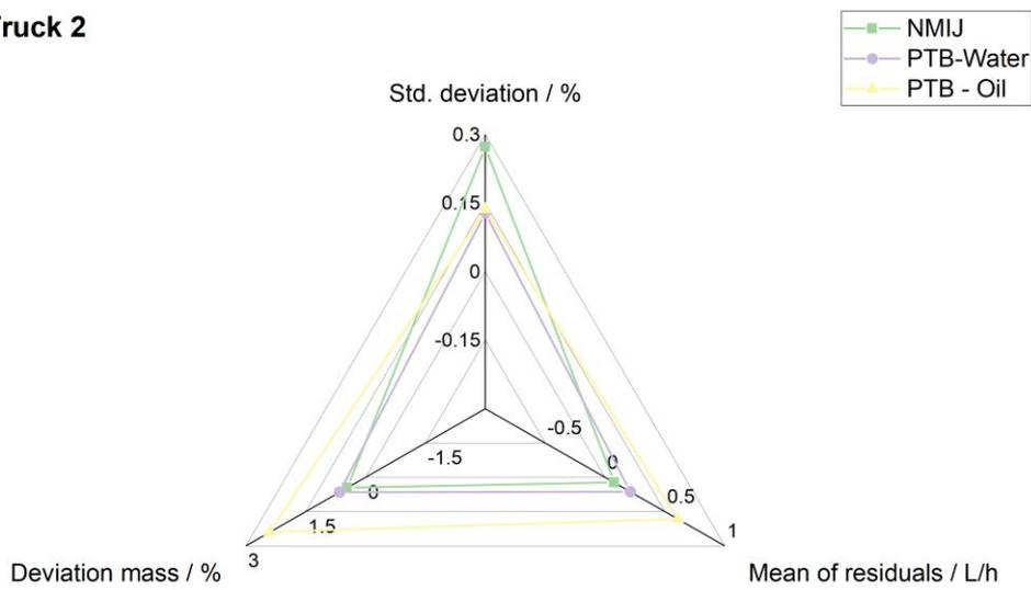
Figure 15: Comparison of the generation of the truck profile 2 based on the mean value of the residuals, the deviation of the mass from the specification and the repeatability.
