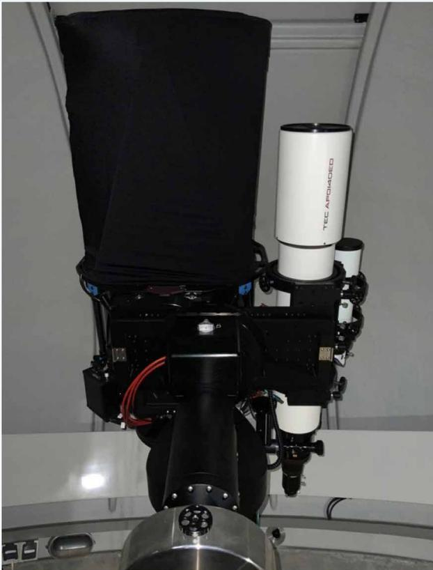
Abb. 2: Teleskop 17'' Plane Wave CDK
