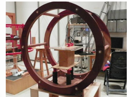
The transfer standard - Garrett coil - with the PTB's free precession NMR-probe inside.
