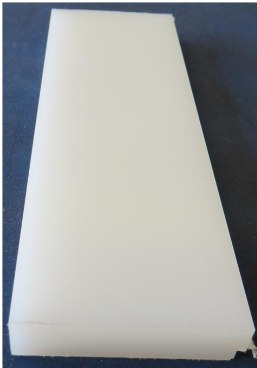
High-density polyethylene (HDPE) with dielectric constant ( \epsilon_r ) : 2.3
