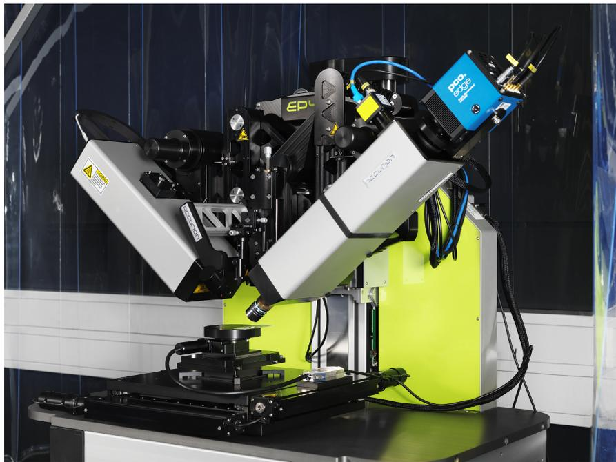
**Figure 3.8** – Custom Accurion EP4 imaging ellipsometer.
