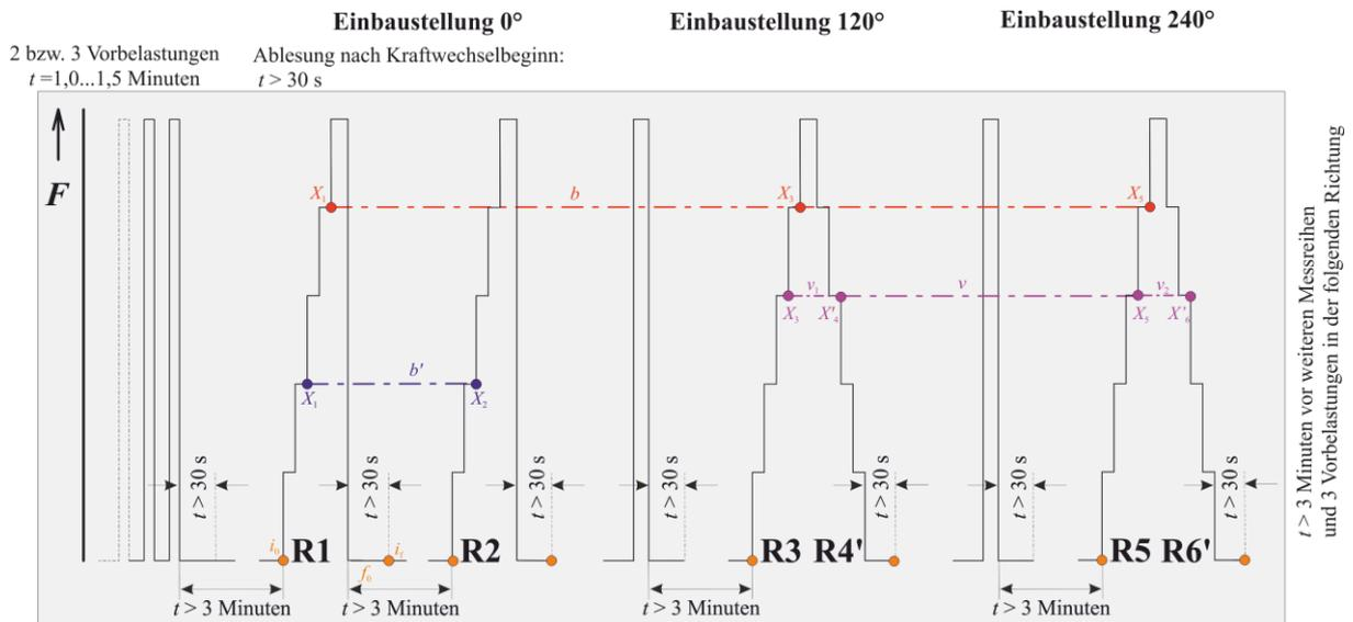
**Figure 4:** Example calibration sequence A; three mounting positions, five force steps
