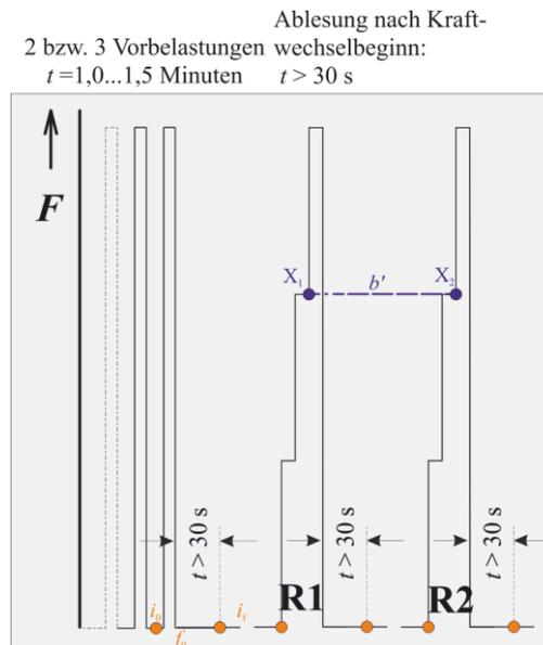
**Figure 7:** Example calibration sequence D; one mounting position, two measurement series, two increasing loadings, three force steps (2 or 3 preloads, reading after start of force change)
