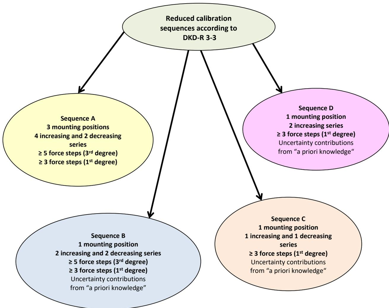
**Figure 3:** Calibration sequences of DKD-R 3-3 including indication of the number of mounting positions, force steps and the usual degree of the regression function
