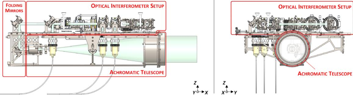
Figure 3. Scale presentation of the mechanical structure of the measurement head. The total length of the head is about 0.75 m. The head is mounted in a protective housing, which allows thermal as well as mechanical decoupling to the optical assembly. A total weight of 45 kg also includes the base for the head.
