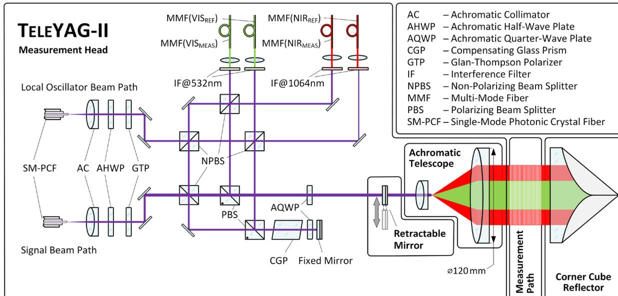
FIGURE 2. Scheme of the optical interferometer principle which was built in the measurement head to form two sub-interferometers. Two SM-PCF guide the frequency-shifted radiation of the multiwavelength laser source to the optical setup. After propagating through the optics, the beams are coupled into four multi-mode fibers to guide the interfered light to the phase evaluation electronics.
