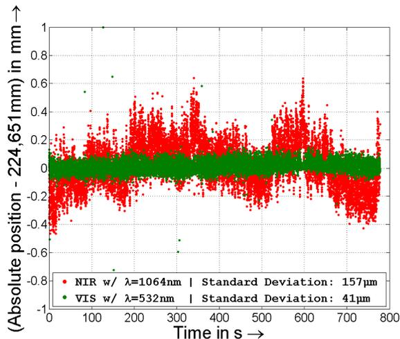
FIGURE 4. Absolute position results at the WUT200 campaign over a distance of 224,651 mm measured with PTB's multi-wavelength interferometer. The standard deviation of  $41 \mu\text{m}$  at 532 nm corresponds to a relative accuracy of  $1.85 \times 10^{-7}$ .
