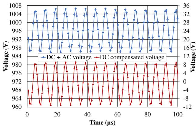
Fig. 12. 1000 V DC signal with added sinusoidal AC signal with an amplitude of 20 V peak to peak at 150 kHz, measured with DC signal (blue) and with compensated DC signal (red)
