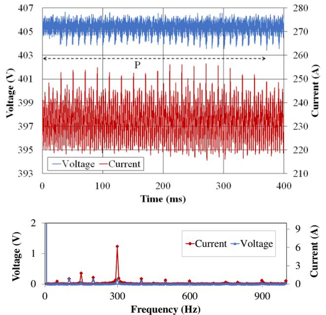
Fig. 7. AC disturbance measured during charging process with combination A1. Lower graph: Spectrum of signals in time period “P”
