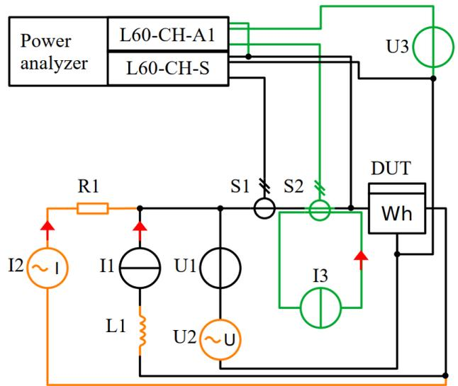
Fig. 10. DC meter testbed. In black are the components necessary for testing DC energy meter with DC phantom power. Orange are the additional components used for the generation of added AC signals. Green are the components to compensate the DC signals for AC measurement
