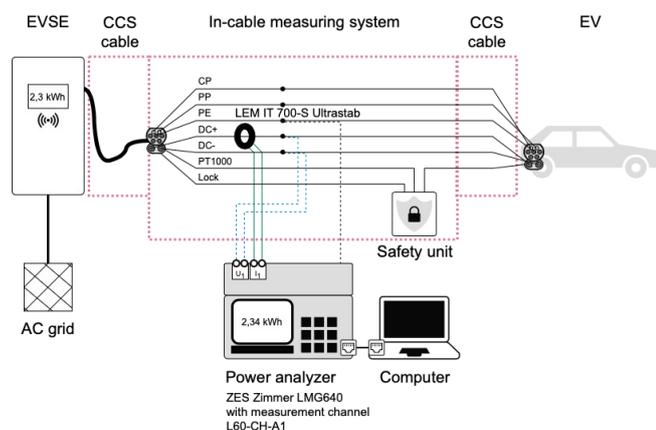
Fig. 1. Measurement setup for onsite measurement at DC charging stations
