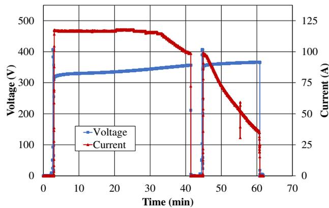
Fig. 6. Voltage and current behavior measured during charging process with combination C3
