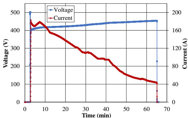
Fig. 3. Voltage and current behavior measured during charging process with combination B1
