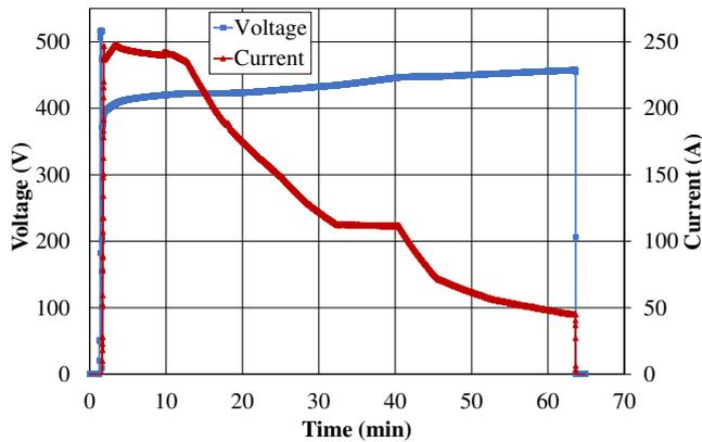
Fig. 5. Voltage and current behavior measured during charging process with combination B3
