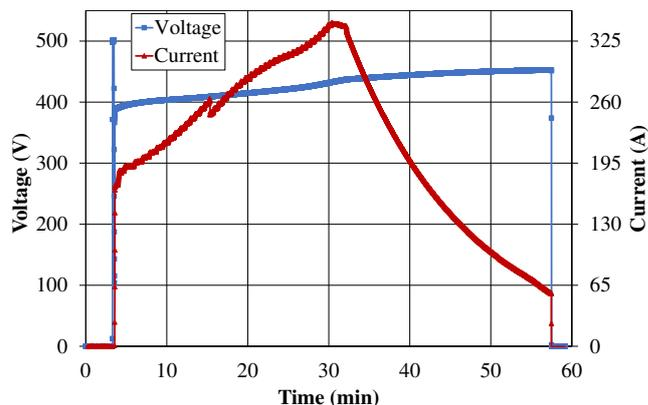
Fig. 2. Voltage and current behavior measured during charging process with combination A1
