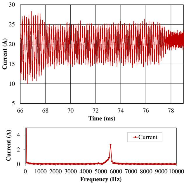
Fig. 9. 5,5 kHz AC disturbance on current signal during the current rise at the beginning of the charging process measured with combination B3. Lower graph: Spectrum of current signal
