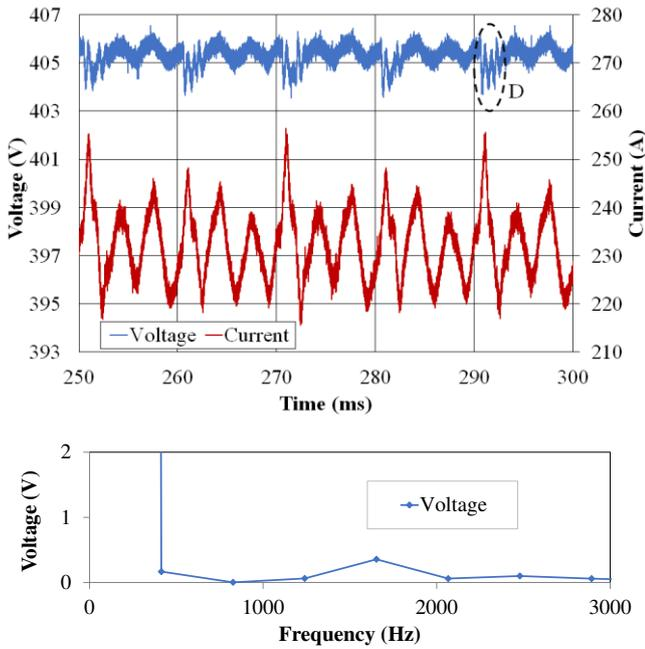
Fig. 8. 300 Hz AC disturbance measured during charging process with combination A1. Lower graph: Spectrum of disturbance "D"
