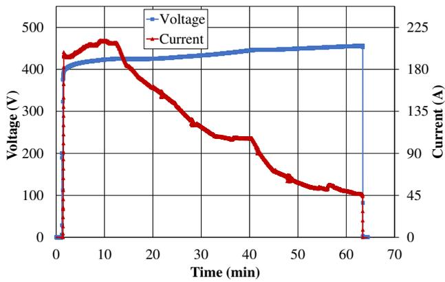
Fig. 4. Voltage and current behavior measured during charging process with combination B2
