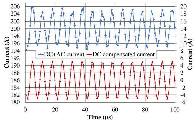
Fig. 11. 200 A DC signal with added sinusoidal AC signal with an amplitude of 10 A peak to peak at 150 kHz, measured with DC signal (blue) and with compensated DC signal (red)
