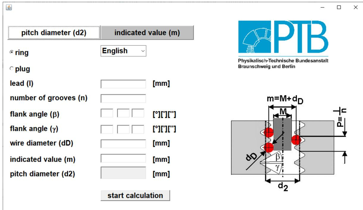
**Figure 13:** Screenshot of the PTB programme (available free of charge) for the exact calculation of the pitch diameter according to Berndt without consideration of the flattening caused by the probing force.
