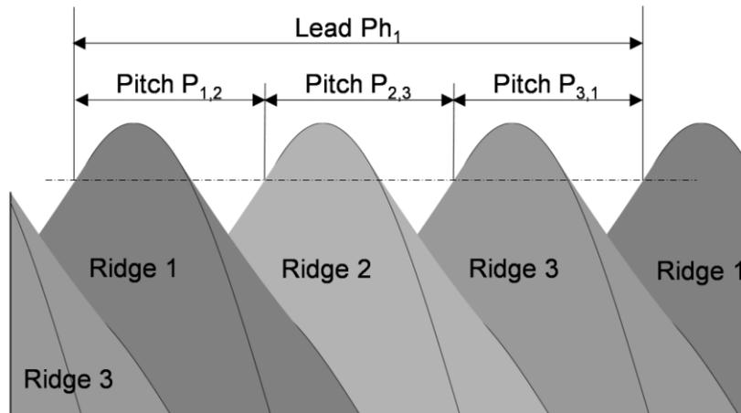
**Figure 3:** Pitch and lead on a three-start external thread. The parameters are only shown for one flank direction. For the flanks in the other direction, additional parameters apply.
