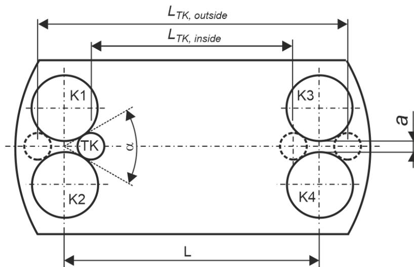
**Figure 16:** Schematic representation of the principle of the gap measurement standard
