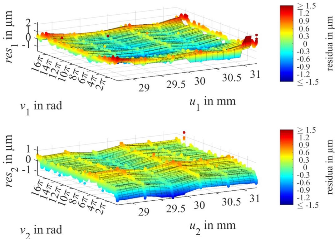
**Figure 8:** Illustration of the measurement result of the areal measurement (developed view of both thread flanks)
