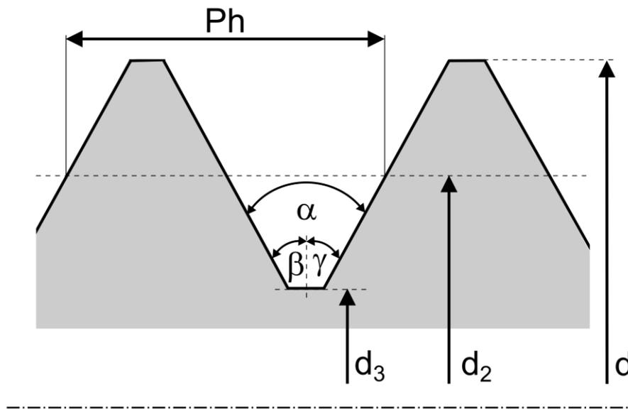
**Figure 2:** Parameters on a single-start external thread according to DIN 2244:2002-05
