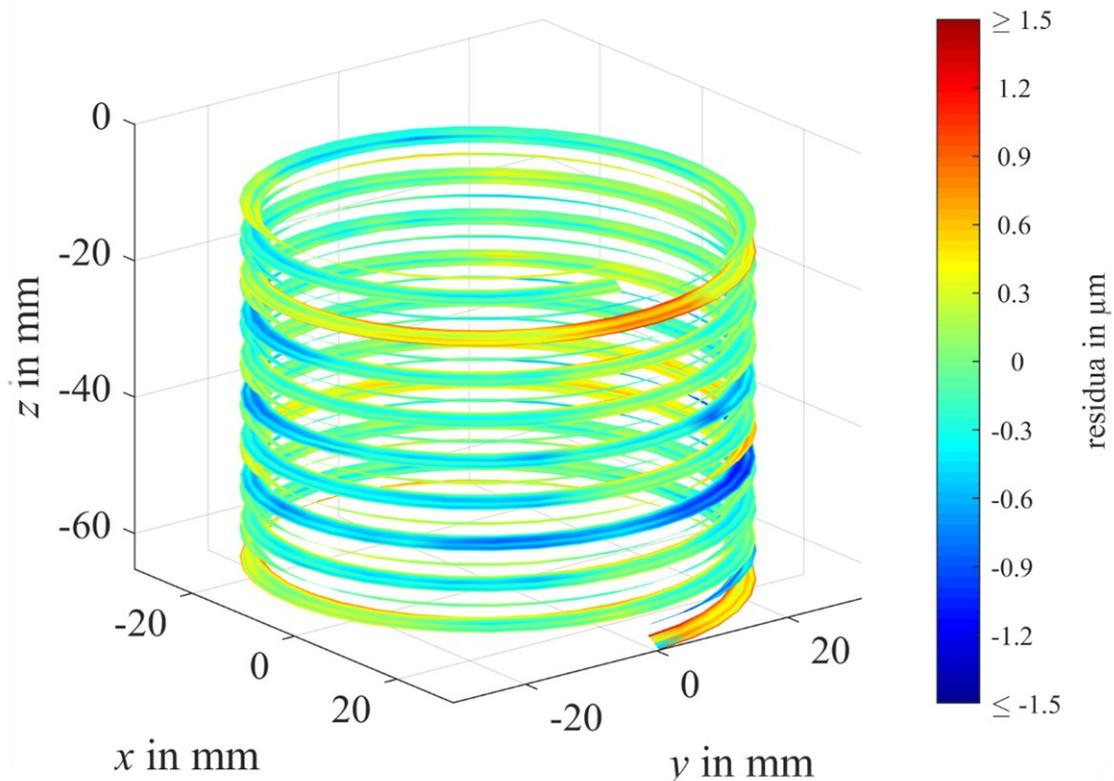
**Figure 7:** Illustration of the result of the areal thread measurement using a Coordinate Measuring Machine (CMM)
