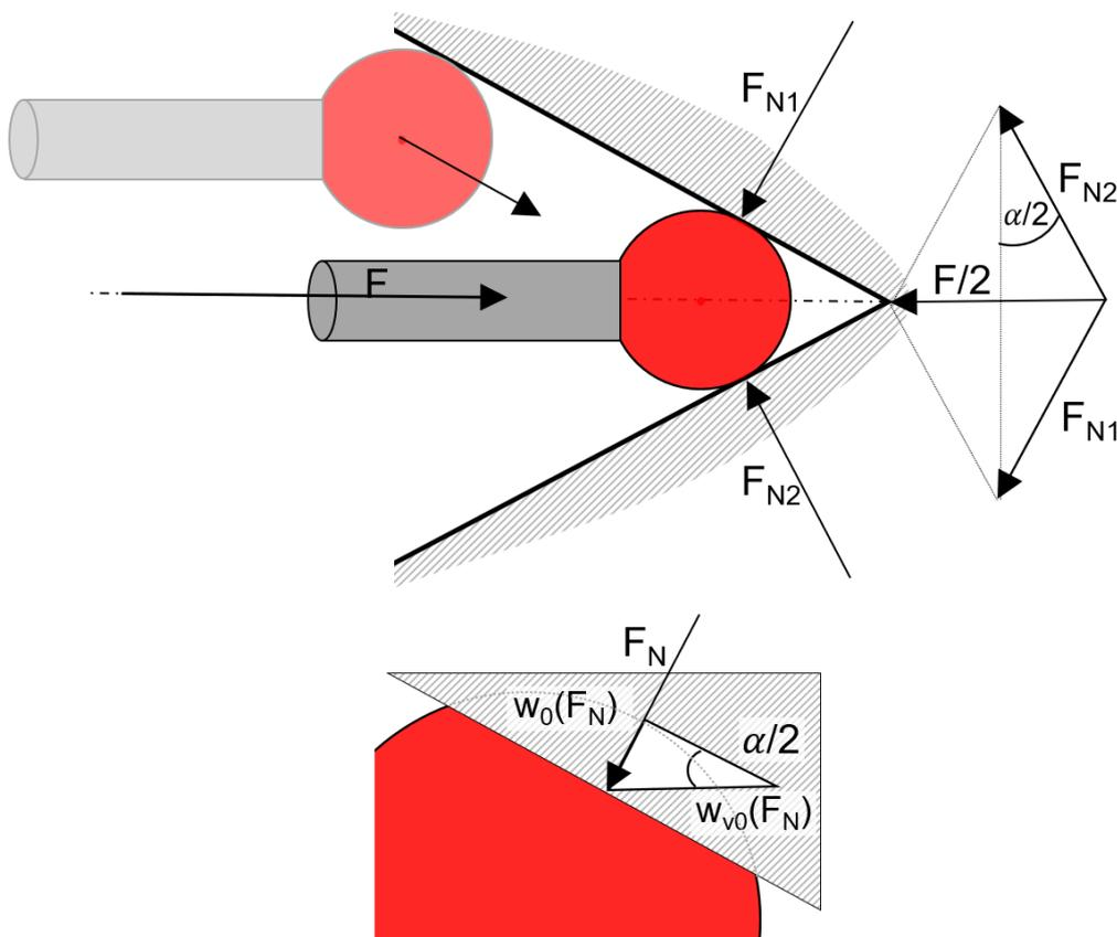
**Figure 14:** Flattening due to wear in two-flank contact
