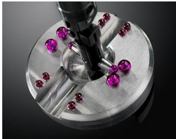
**Figure 17:** Example of a gap measurement standard
