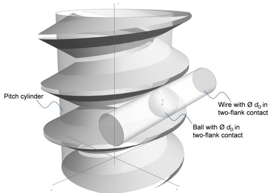
**Figure 10:** Measuring wire and ball in two-flank contact on the pitch diameter of a symmetrical external thread. The contact points of wire and ball are identical and lie in a normal section of the thread.
