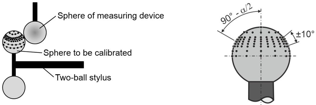
**Figure 15:** Pattern (calibration points) for calibrating screw thread probe balls
