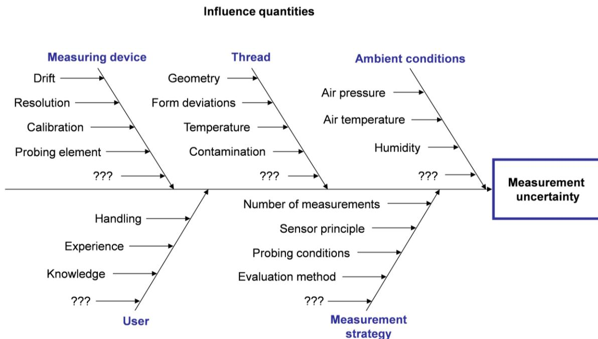
**Figure 9:** Ishikawa diagram to illustrate the influence quantities acting on the measurement process
