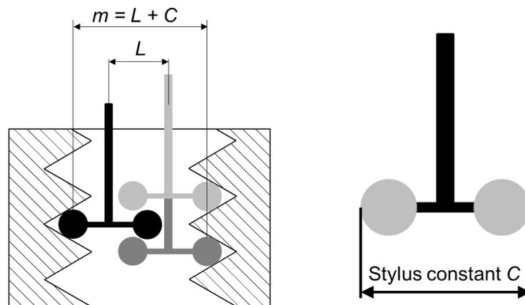
**Figure 5:** Measurement of the indicated value  $m$  on a single-start internal thread using the two-ball method
