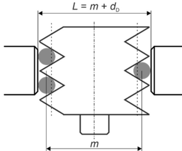
**Figure 4:** Measurement of the indicated value  $m$  on a single-start external thread using the three-wire method
