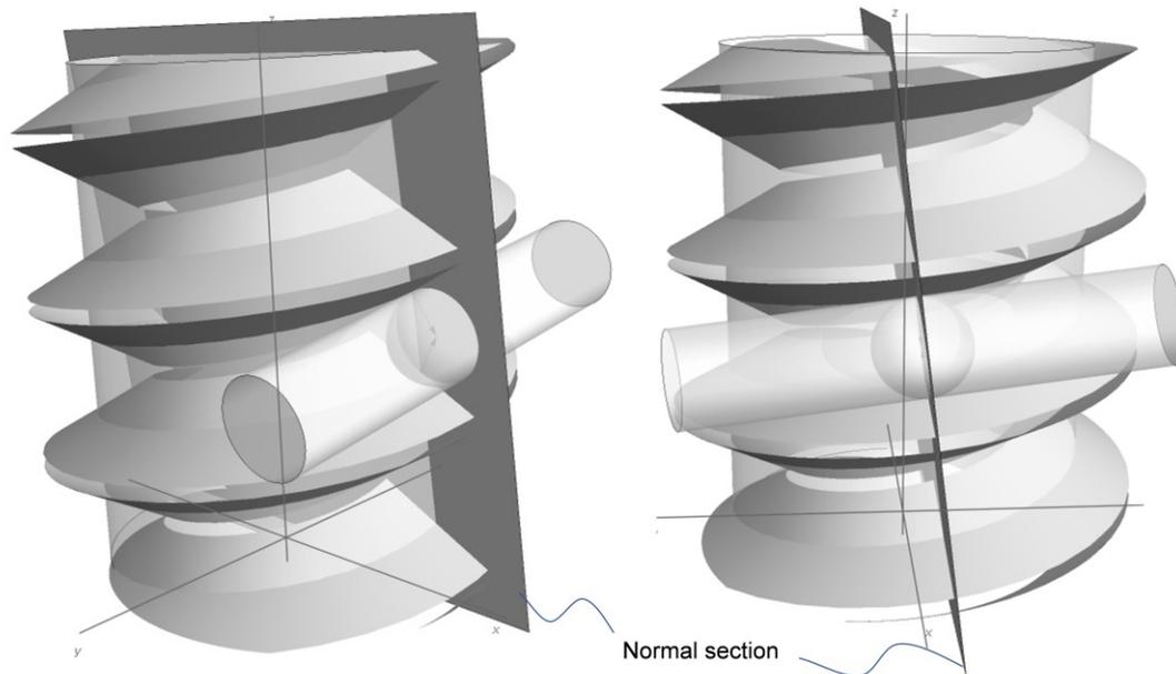
**Figure 11:** Illustrated are two views of the same figure already depicted in Figure 10; here, the normal section belonging to the contact points has been added. In the right-hand view it can be clearly seen that the contact points of the ball and wire lie in this normal section and that this plane is inclined with respect to the axial section through the centre of the ball, which contains the z-axis.
