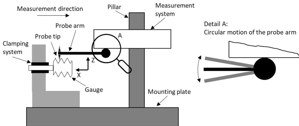
**Figure 6:** Measurement of a single-start external thread on a stylus instrument
