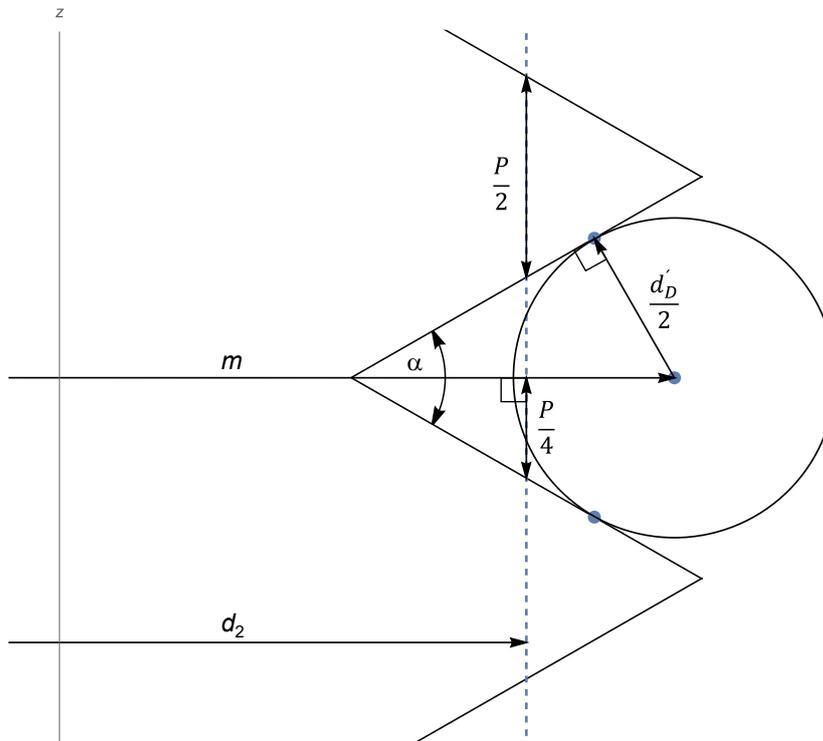
**Figure 12:** An infinitely thin circular disc with diameter  $d'_D$  touches both flanks of the thread in the same axial section. Here, the pitch diameter  $d_2$  results from the indicated value  $m$  by simple trigonometric calculations in the two right-angled triangles shown.
