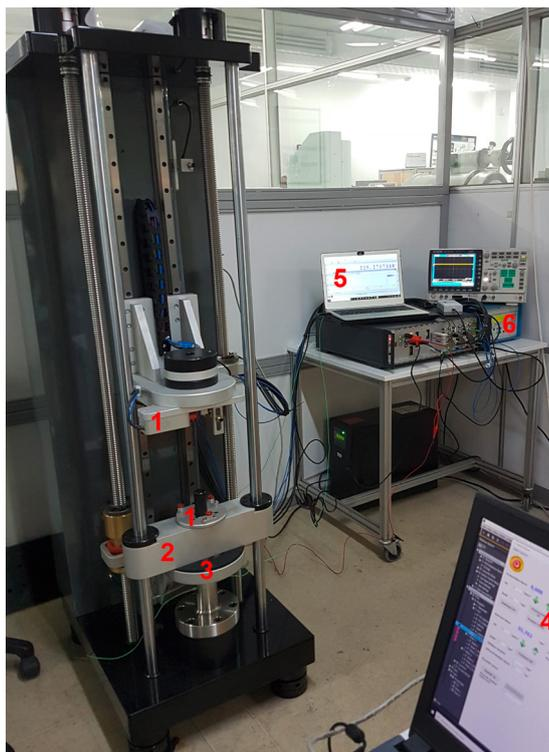
Figure 7: Developed dynamic pressure calibration system.
