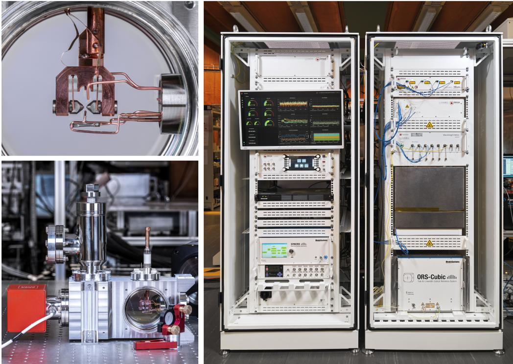
Figure 2.7: **Setup of opticlock.** Top left is a picture of the trap, identical to the Yb3 design but without the gold-coating on the endcap electrodes. Bottom left shows the vacuum chamber with installed trap. The right hand side picture is a view of the full setup. The left rack houses the electronic components, the right rack contains lasers, cavity and the physics package.
