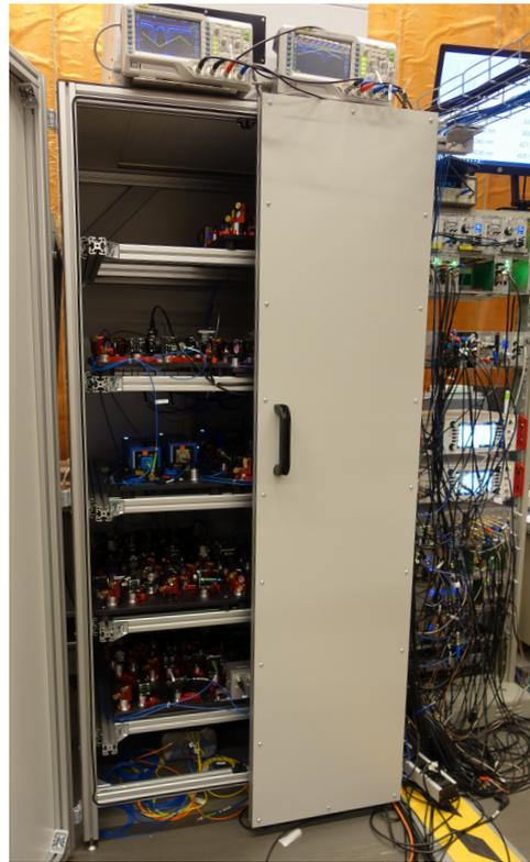
Figure 2.6: **Laser cabinet** with individually extractable platforms for optical breadboards.
