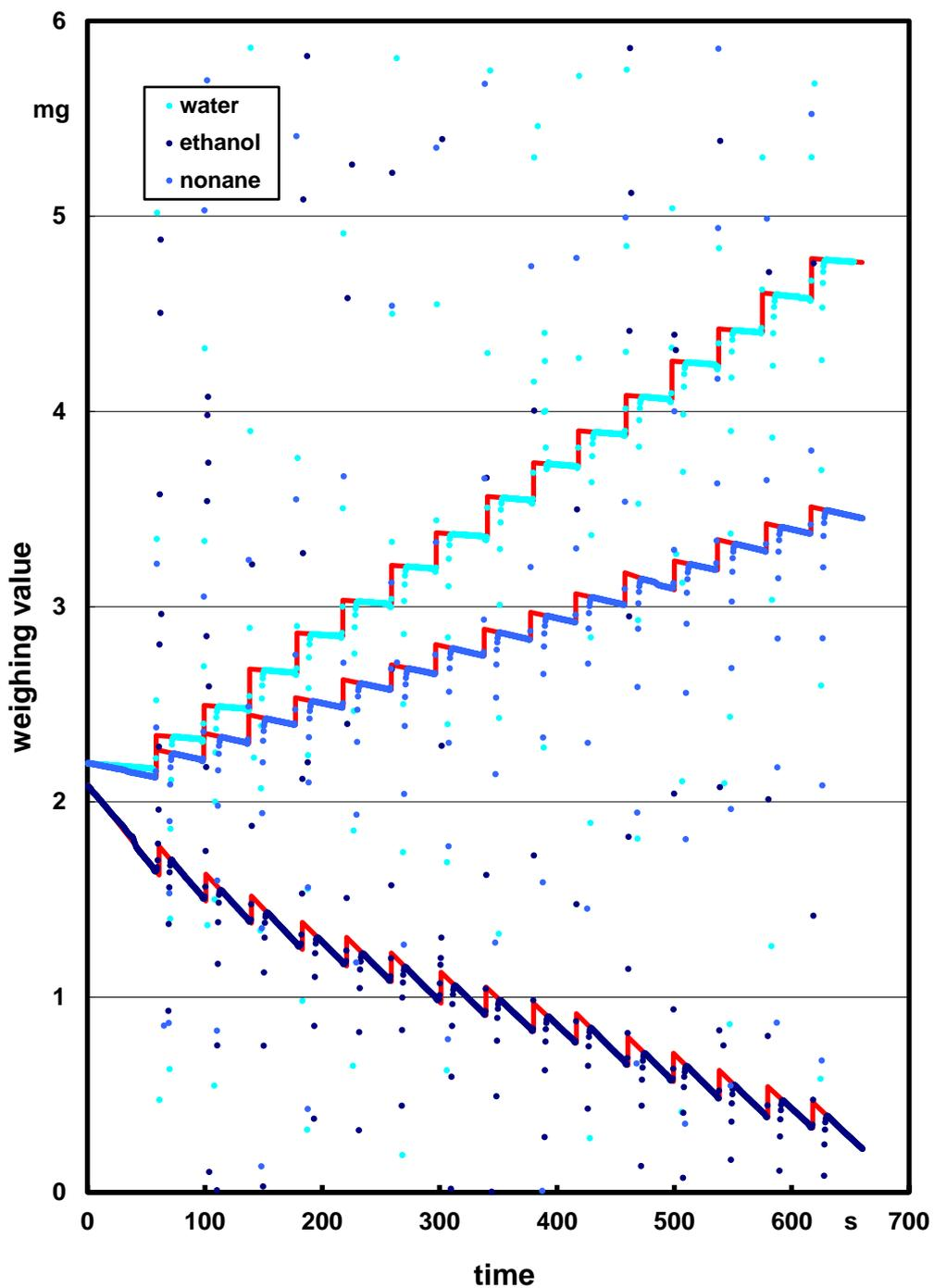
Fig. 15: Weighing value for 15 dispensing operations of 0.2  $\mu\text{l}$  water, ethanol and nonane, respectively, with a microlitre syringe. The continuous step curves are composed of regression lines. The leap onto the next line occurs at the moment of each dispensing operation. The height of the steps is a measure of the respective weighing value of the dispensed volume.
