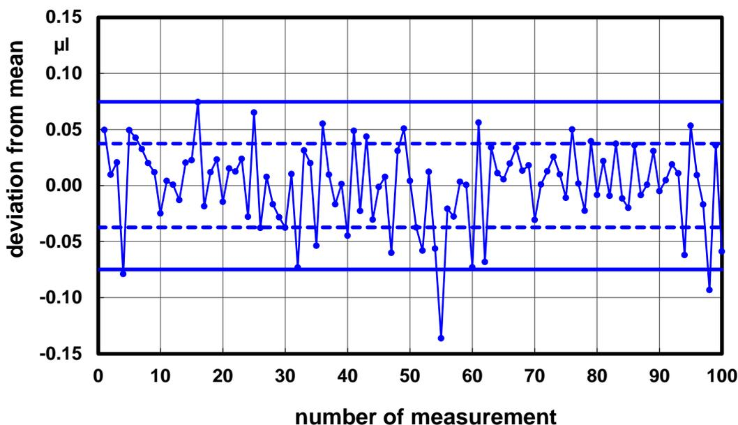
Fig. 37: Dispensing of water repeated 100 times. Positive displacement piston-operated pipette with a test volume of 10  $\mu\text{l}$ . The values plotted are the deviation of the individual measurements from the average of all measurements. The dashed line shows the simple standard deviation determined for all of the 100 measurements ( $k = 1$ ); the solid line shows the expanded standard deviation ( $k = 2$ ).
