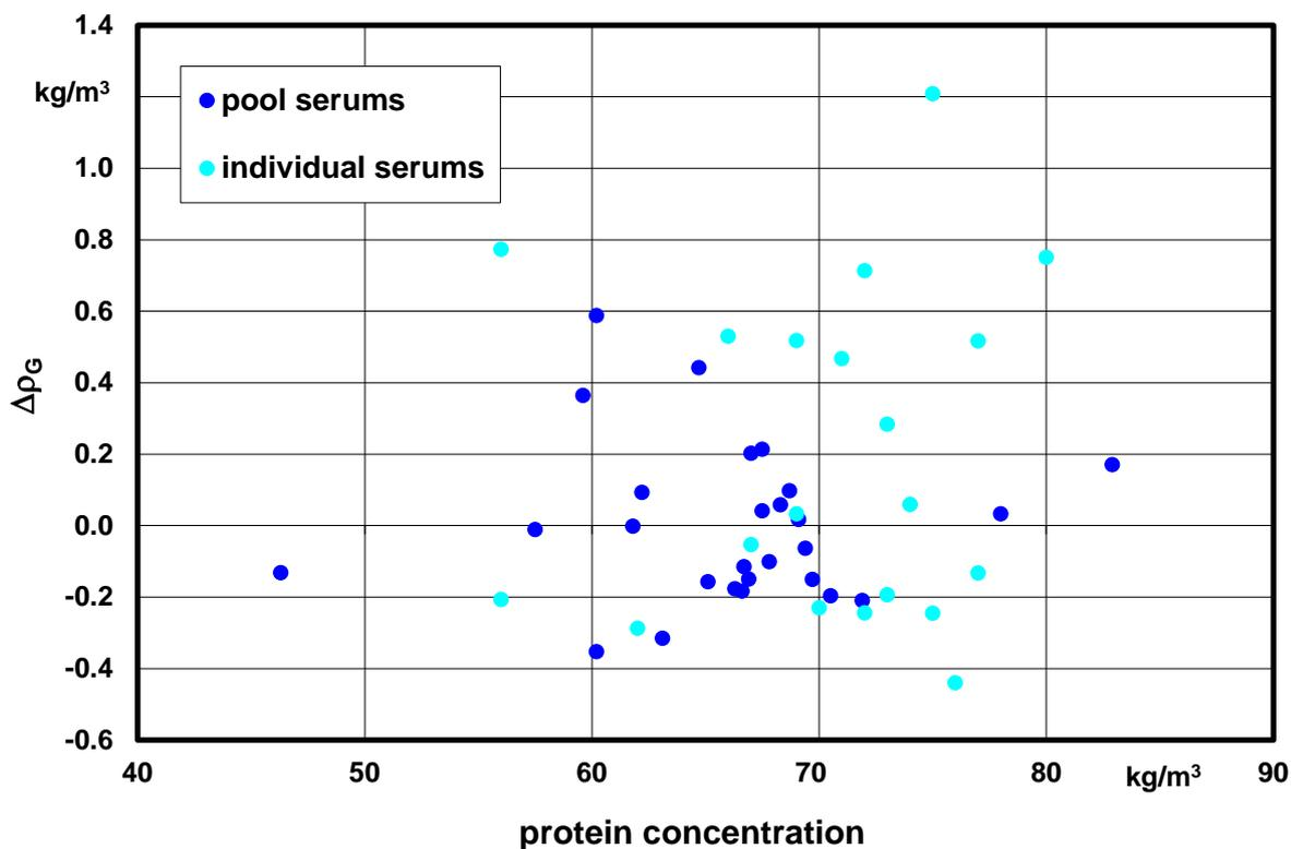
Fig. 35: Comparison of the density of individual serums and of pool serums
