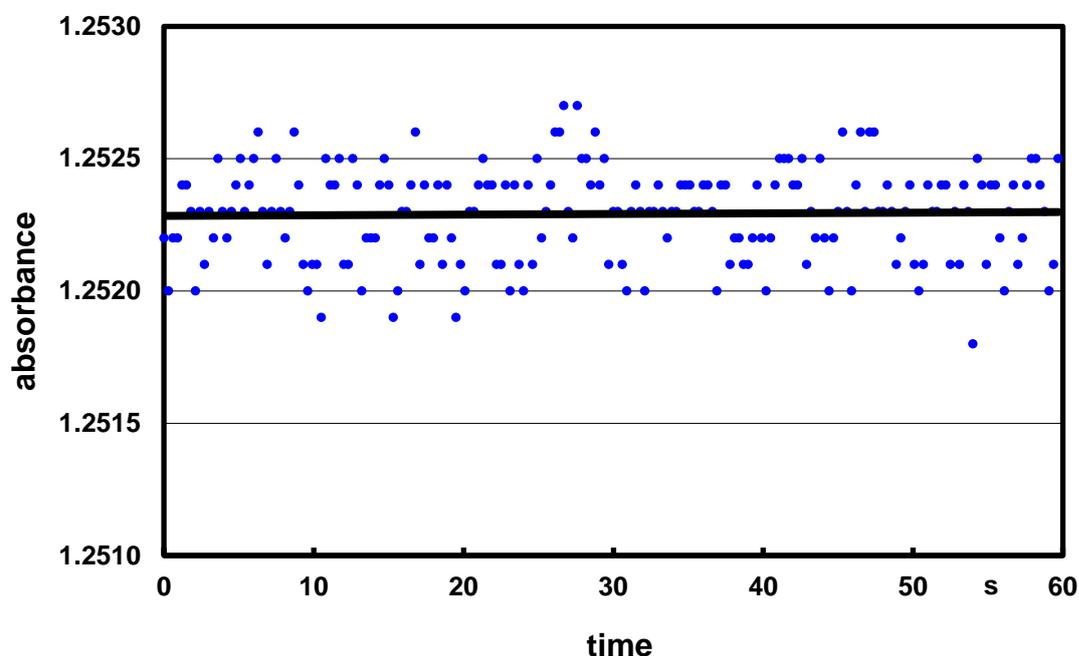
Fig. 44: Measured absorbance of a dispensing of 10  $\mu\text{l}$  of contrast agent solution in 1.3 ml of water. The straight line plotted is fitted to the measurement data by means of a linear regression. It shows the time drift of absorbance from 1.252283 to 1.252298 after 60 s. The resolution of the photometer is 0.0001. The drift is therefore negligible within the limits of the measurement uncertainty.
