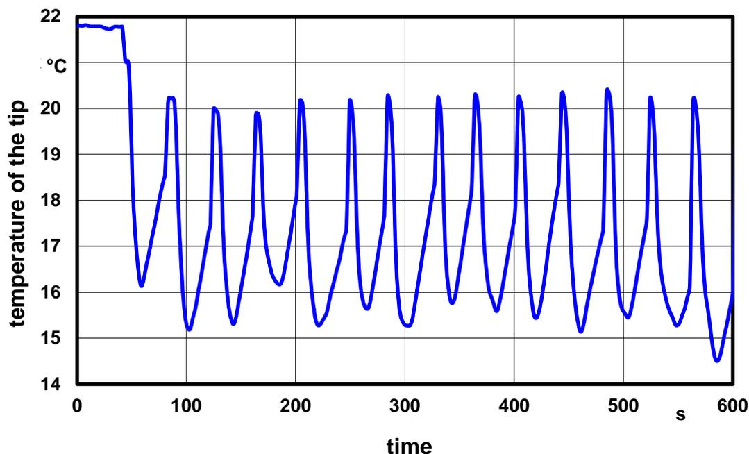
Fig. 10: Temperature behaviour of a pipette tip after filling it and expelling the liquid (using ethanol); cycle consisting of 14 individual dispensing operations.
