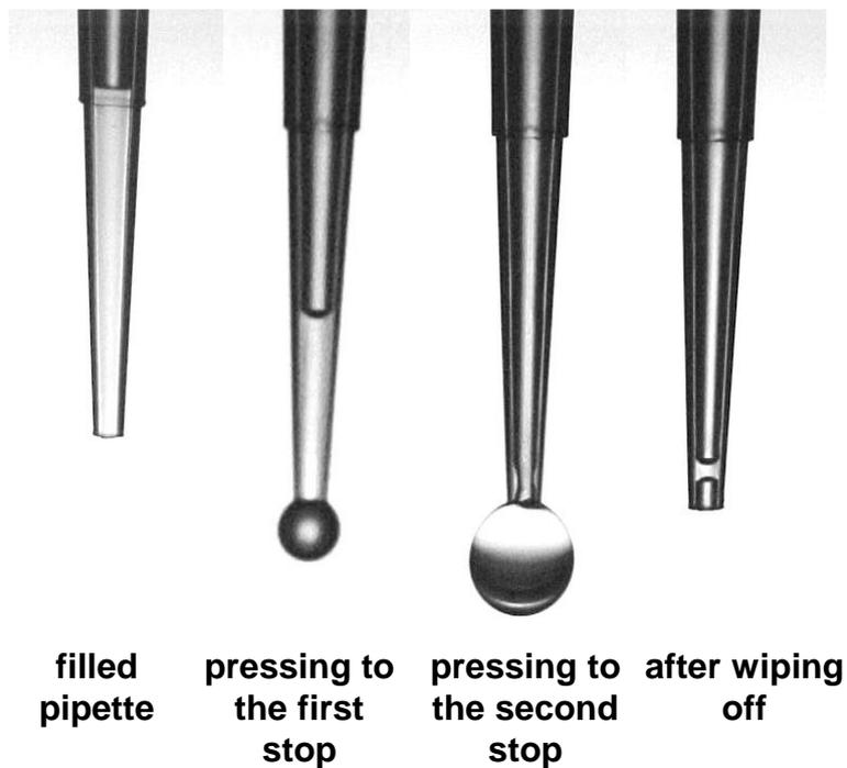
Fig. 22: Sequence of pictures showing the tip of an air displacement pipette filled with **serum** being emptied. The quantity of liquid is 2  $\mu\text{l}$ . For the purpose of these photos, the pipette tip was not drawn against the wall of the vessel.
