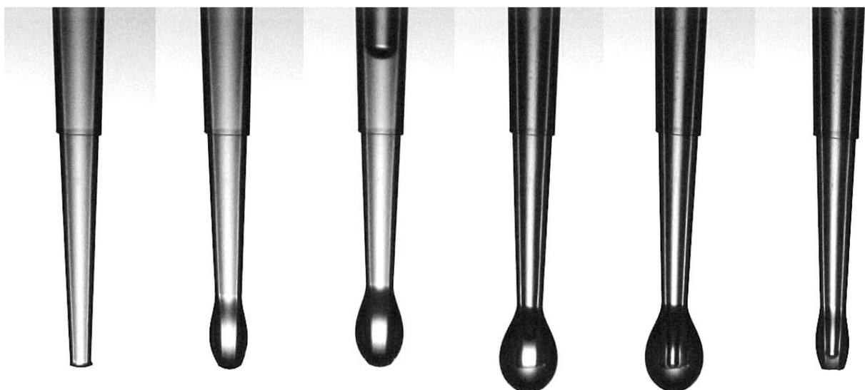
Fig. 20: Wettability of the pipette tip while expelling nonane. For the purpose of these photos, the pipette tip was not drawn against the wall of the vessel.
