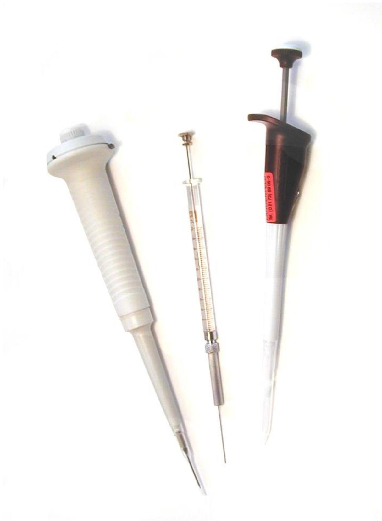
Volumetric apparatus for the dispensing of liquids in the microlitre range
