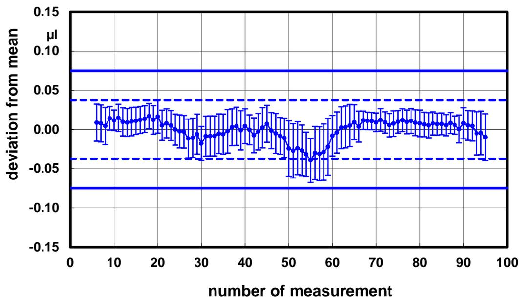
Fig. 38: Dispensing of water repeated 100 times. Floating average with averaging across 10 individual dispensing operations each time. The values plotted are the deviation of the 10 average values from the average of all measurements. The data of the individual measurements are plotted in Fig. 37. The dashed line shows the simple standard deviation determined for all of the 100 measurements ( $k = 1$ ); the solid line shows the expanded standard deviation ( $k = 2$ ).
