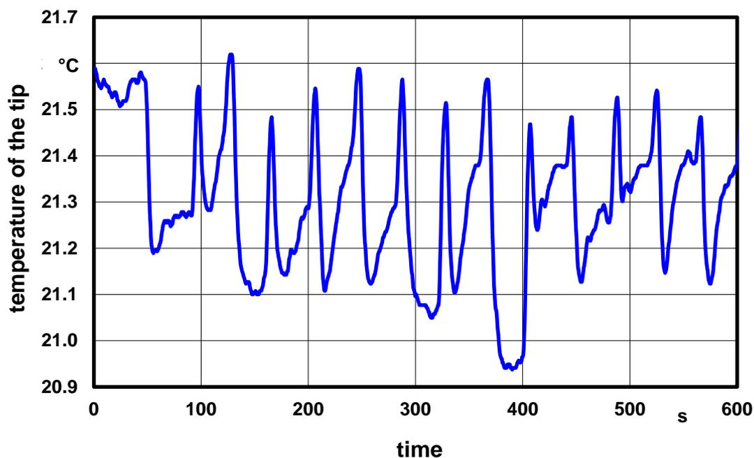
Fig. 9: Temperature behaviour of a pipette tip after filling it with water and after expelling the liquid; cycle consisting of 14 individual dispensing operations.
