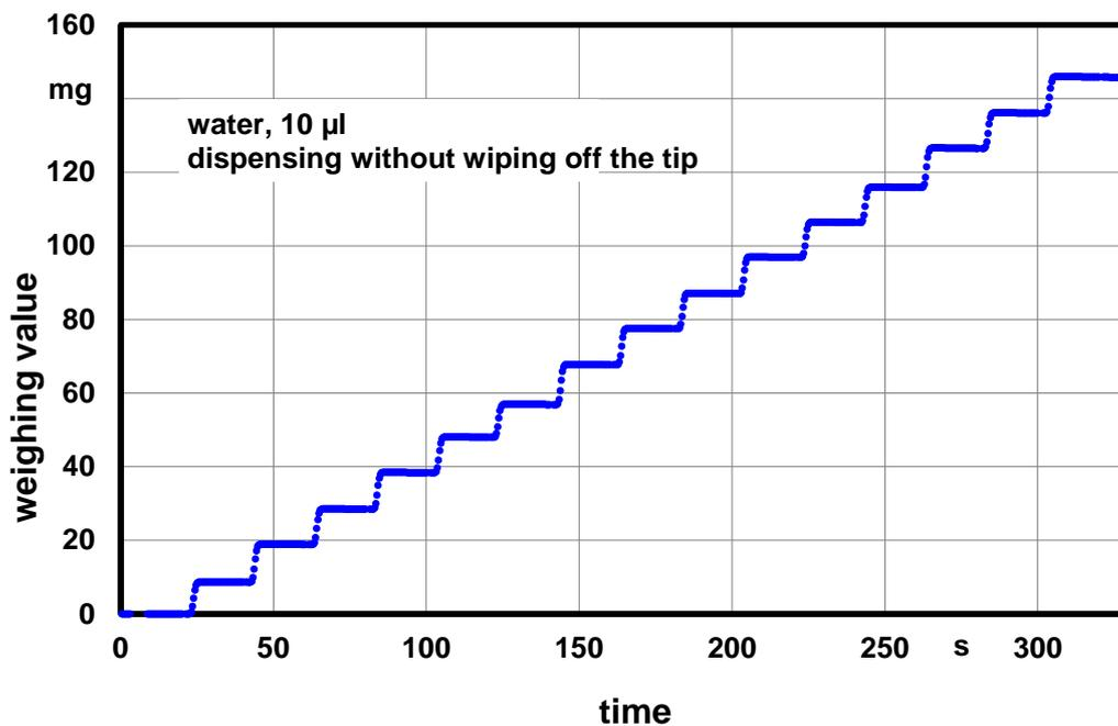
Fig. 4: Weighing value as a function of time for measurements including 15 dispensing operations of 10 µl water each, **without** wiping off the tip. The time interval between the individual dispensing operations is reduced to 20 s. Each interval between the measurement points amounts to 0.4 s.
