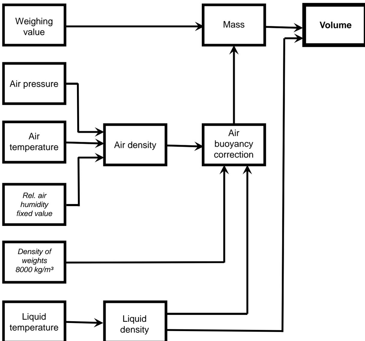
Fig. 1: Flow chart on the relations between the quantities required to determine volume gravimetrically. The boxes in italic font contain fixed values that are used instead of measured values.
