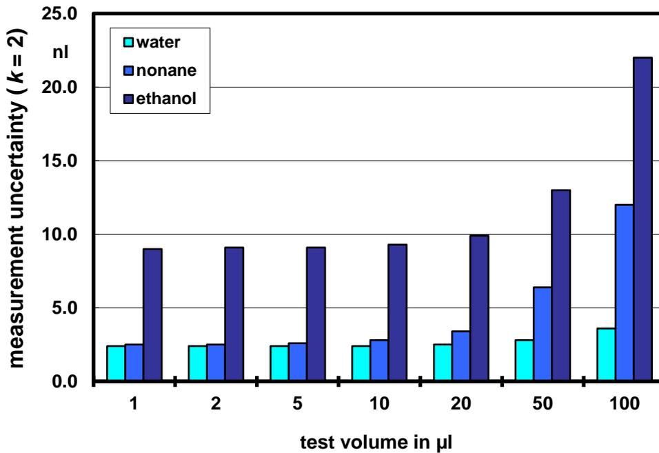
Fig. 11: Expanded measurement uncertainty ( $k = 2$ ) for the measurement of liquid volumes using the gravimetric measuring setup for selected test volumes. In the case of volumes smaller than  $10 \mu\text{l}$ , the measurement uncertainty is practically independent of the volume measured.
