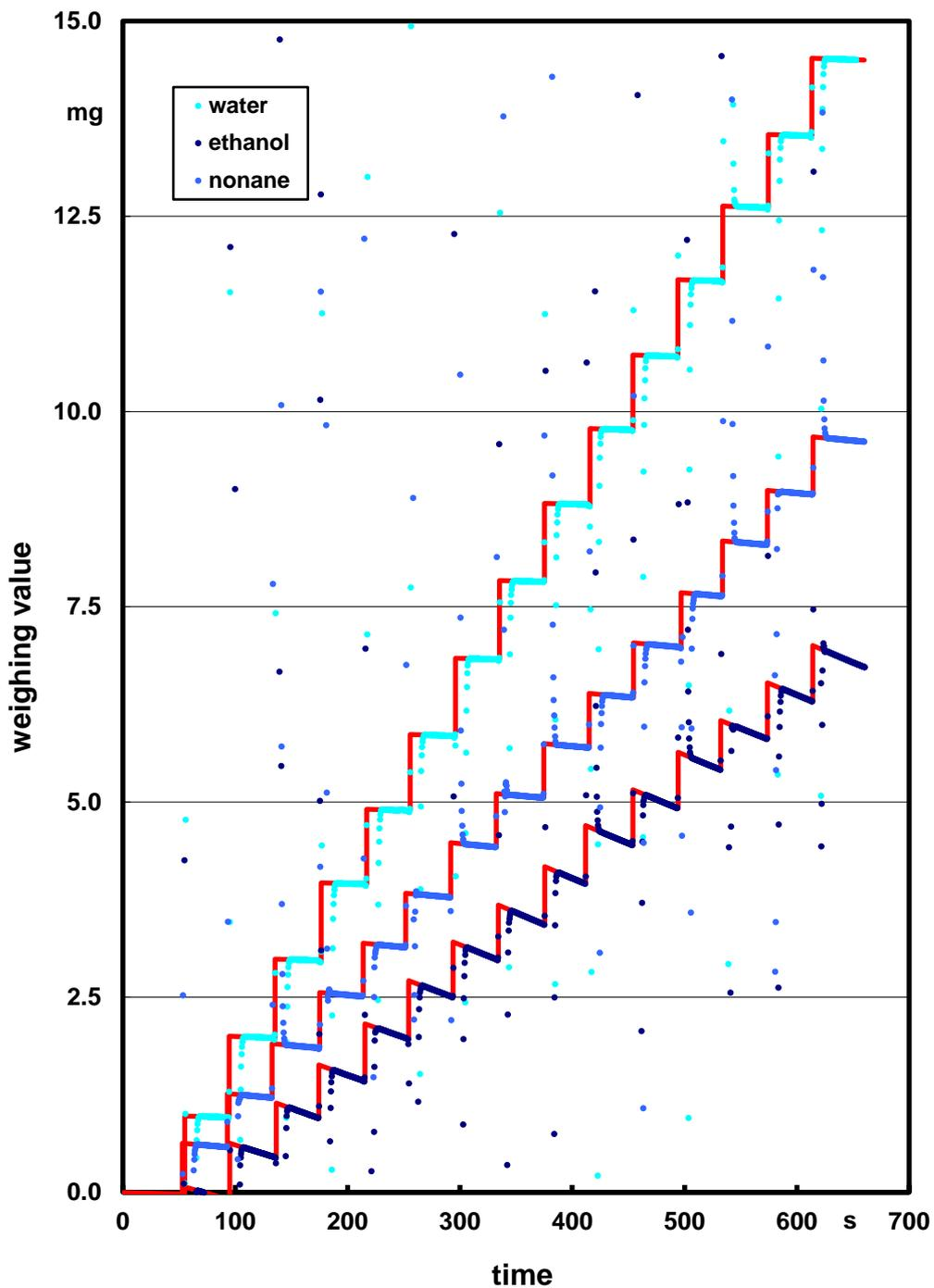
Fig. 14: Weighing value for 15 dispensing operations of 1  $\mu\text{l}$  water, ethanol and nonane, respectively, with a positive displacement piston-operated pipette with a plastic piston and a plastic cylinder. The continuous step curves are composed of regression lines. The leap onto the next line occurs at the moment of each dispensing operation. The height of the steps is a measure of the respective weighing value of the dispensed volume.
