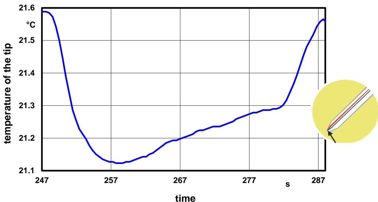
Fig. 8: Temperature behaviour of a pipette tip after filling it with water and after expelling the liquid. The insert on the right is a schematic description of the arrangement of the temperature sensor in the pipette tip.
