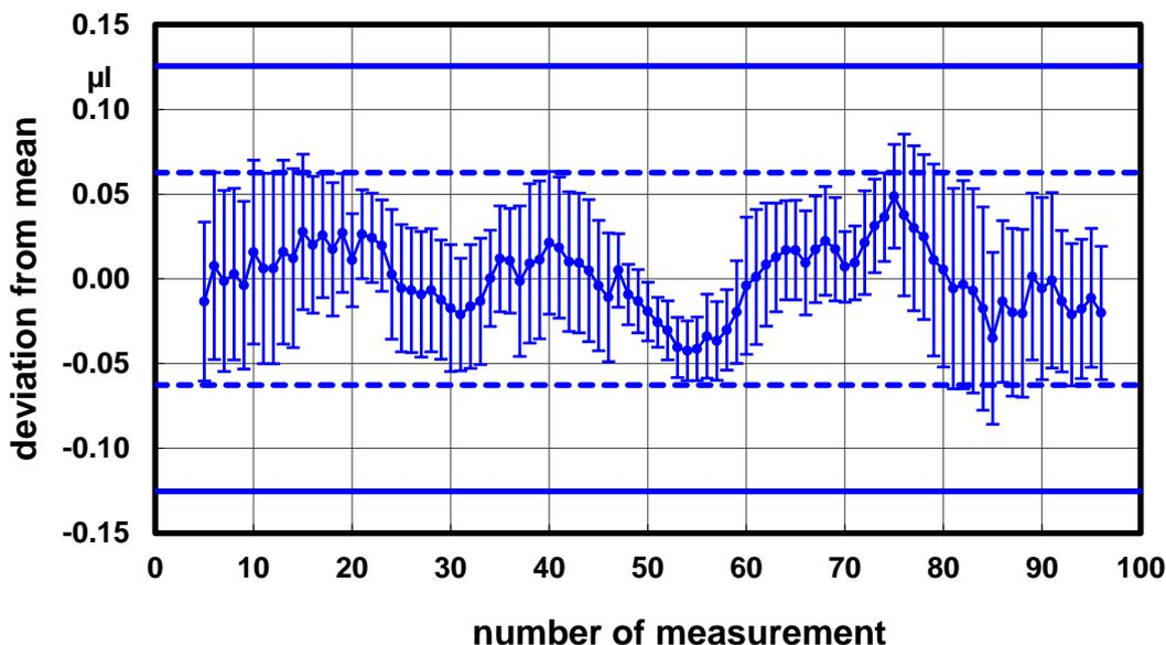
Fig. 40: Dispensing of serum repeated 100 times. Floating average with averaging across 10 individual dispensing operations each time. The values plotted are the deviation of the 10 average values from the average of all measurements. The data of the individual measurements are plotted in Fig. 39. The dashed line shows the simple standard deviation determined for all of the 100 measurements ( $k = 1$ ); the solid line shows the expanded standard deviation ( $k = 2$ ).
