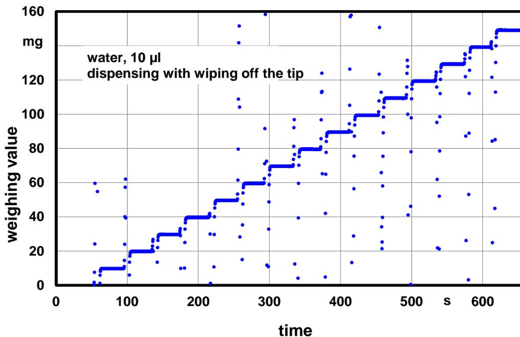
Fig. 5: Weighing value as a function of time for measurements including 15 dispensing operations of 10 µl water each, **wiping off** the tip. The time interval between the individual dispensing operations amounts to 40 s. Each interval between the measurement points amounts to 0.4 s. The scattering of the measured values immediately after each dispensing operation is explained in the text.
