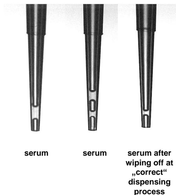
Fig. 23: Serum remaining in the pipette tip after the dispensing. The original quantity of liquid was 2  $\mu\text{l}$ . During the dispensing in the picture on the right, the pipette tip touched the vessel inner wall; this was not the case in the picture on the left and in the one in the middle.
