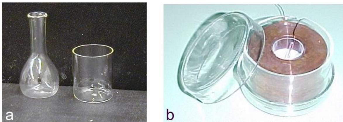
Fig. 3: a) Handmade glass vessels used as the reservoir and the weighing vessel for the liquid. b) Glass vessel with a copper ring for thermal stabilization of the liquid reservoir. Inside the glass vessel: the thermistor used to determine the temperature.
