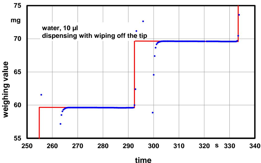
Fig. 6: Section of Fig. 5 with straight fitting lines. The height of the vertical sections is a measure of the weighing value of the dispensed liquid. The recovery time of the balance across which extrapolation must take place is clearly to be seen.
