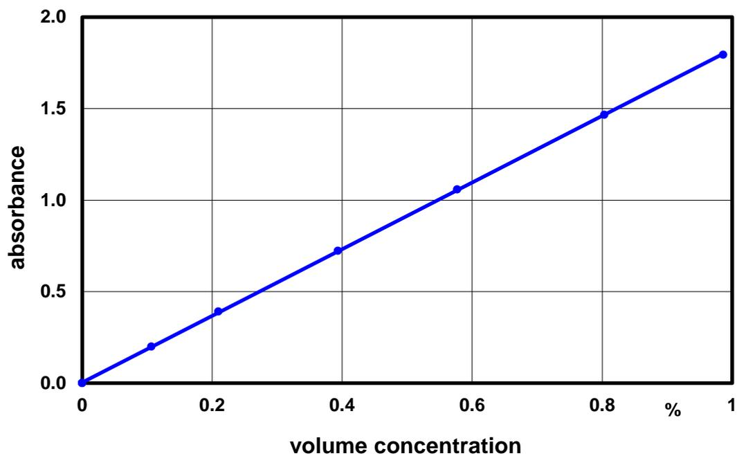
Fig. 43: Calibration curve used to verify Beer's law for a solution of ABTS in **serum**. The area represented is the linear area prevailing for volume concentrations  $c < 1\%$ .
