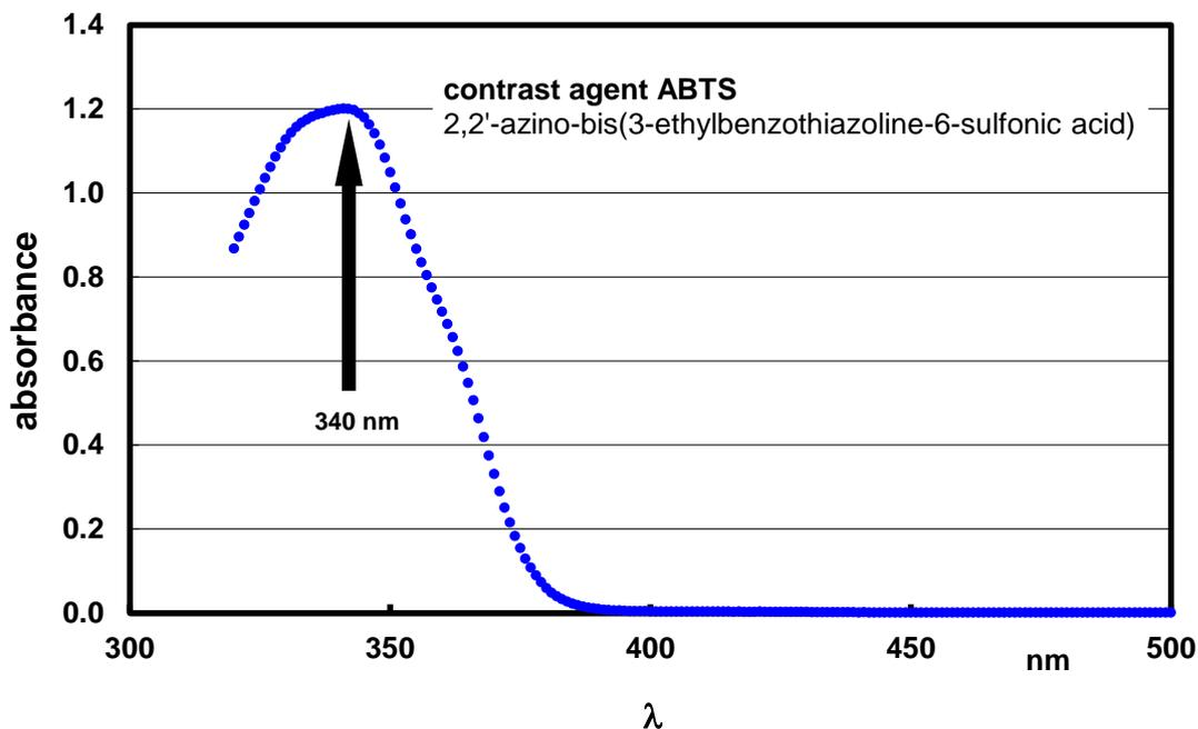
Fig. 41: Absorption spectrum of the contrast agent used (ABTS). The absorption maximum is 340 nm. This wavelength was used for the photometric investigations.
