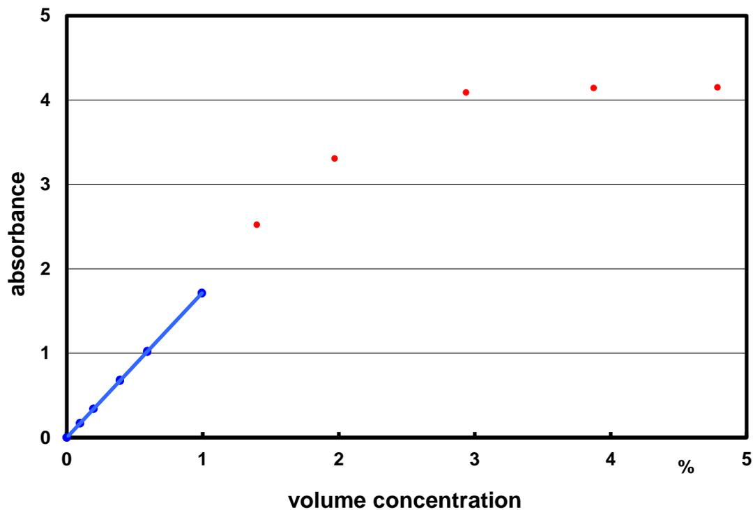
Fig. 42: Calibration curve used to verify Beer's law for a solution of ABTS in **water**. In the lower range, there is a linear correlation between absorbance and the concentration of the contrast agent solution.
