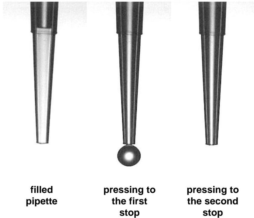
Fig. 21: Sequence of pictures showing the tip of an air displacement pipette filled with **water** being emptied. The quantity of liquid is 2  $\mu\text{l}$ . For the purpose of these photos, the pipette tip was not drawn against the wall of the vessel.
