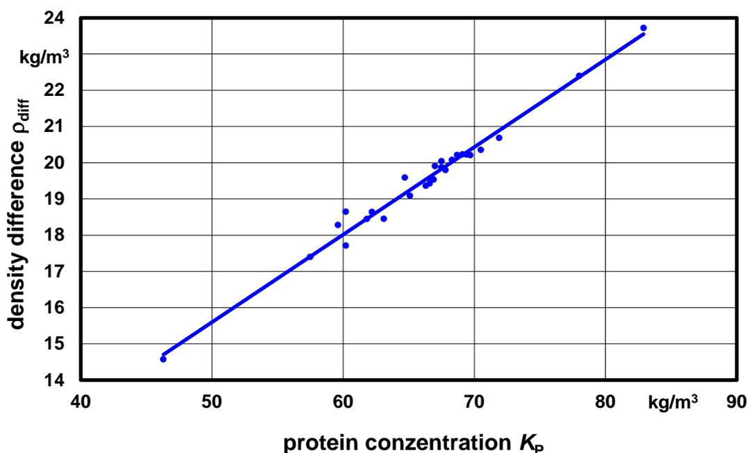
Fig. 34: Density difference  $\rho_{diff}$  of the pool serums investigated as a function of the protein concentration, and accordingly fitted straight lines. See text for the uncertainty of the straight lines.
