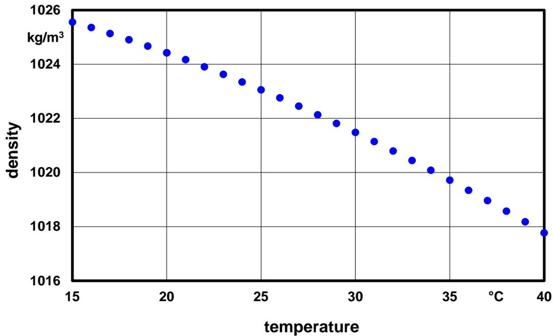
Fig. 36: Temperature dependence of the density of human serum. The shape of the curve is described quantitatively in Equation (10-10).
