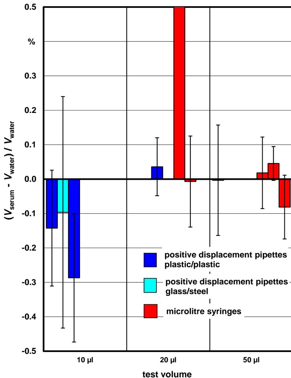
Fig. 25: Difference between the dispensed volume of water and serum for test volumes of 10 µl, 20 µl, and 50 µl. The figure shows the relative difference of the values averaged from 10 dispensing operations for water and for serum, respectively. Each bar represents the results for one dispensing device. The measurement uncertainty bars indicate the uncertainty of the difference which was calculated from the repeatability standard deviation of the relative difference (coverage factor  $k = 2$ ).
