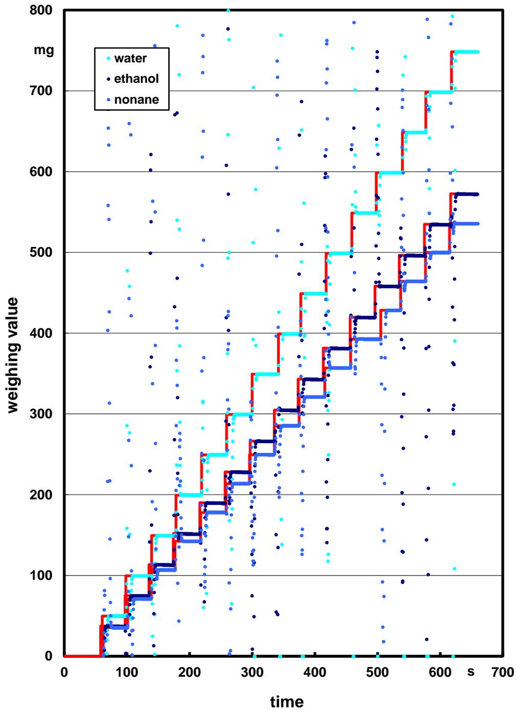
Fig. 12: Weighing value for 15 dispensing operations of 50  $\mu\text{l}$  water, ethanol and nonane, respectively, with a positive displacement piston-operated pipette with a plastic piston and a plastic cylinder. The continuous step curves are composed of regression lines. The leap onto the next line occurs at the moment of each dispensing operation. The height of the steps is a measure of the respective weighing value of the dispensed volume.
