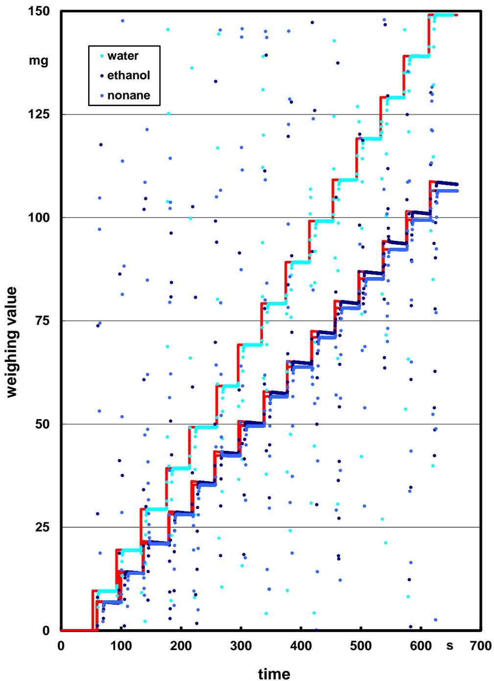
Fig. 13: Weighing value for 15 dispensing operations of 10  $\mu\text{l}$  water, ethanol and nonane, respectively, with a positive displacement piston-operated pipette with a steel piston and a glass cylinder. The continuous step curves are composed of regression lines. The leap onto the next line occurs at the moment of each dispensing operation. The height of the steps is a measure of the respective weighing value of the dispensed volume.
