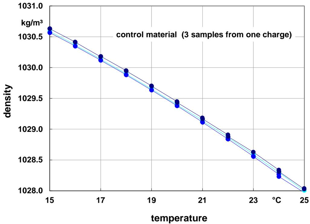
Fig. 30: Temperature-density curve for three control materials reconstituted from material from the same batch (from the same pool)
