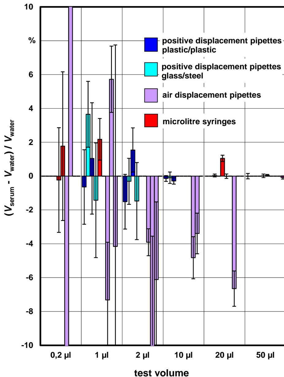
Fig. 27: Difference between the dispensed volume of water and serum for test volumes from 0.2  $\mu\text{l}$  to 50  $\mu\text{l}$ .
