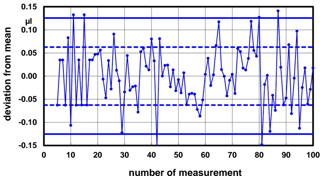
Fig. 39: Dispensing of serum repeated 100 times. Positive displacement piston-operated pipette with a test volume of 10 µl. The values plotted are the deviation of the individual measurements from the average of all measurements. The dashed line shows the simple standard deviation determined for all of the 100 measurements ( $k = 1$ ); the solid line shows the expanded standard deviation ( $k = 2$ ).
