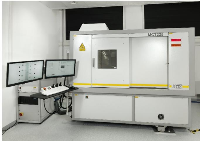
Fig. 3.22. PTB's Nikon Metrology MCT 225 system used for the experiments.
