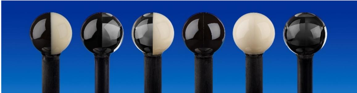
Fig. 3.7. Set of multi- and mono-material compound spheres used for the assessment of the *P*-test. From left to right: three MuMat-spheres Al<sub>2</sub>O<sub>3</sub> & Si<sub>3</sub>N<sub>4</sub>, Si<sub>3</sub>N<sub>4</sub> & N-SF6 and Al<sub>2</sub>O<sub>3</sub> & N-SF6; and three MoMat-spheres Si<sub>3</sub>N<sub>4</sub> & Si<sub>3</sub>N<sub>4</sub>, Al<sub>2</sub>O<sub>3</sub> & Al<sub>2</sub>O<sub>3</sub> and N-SF6 & N-SF6.
