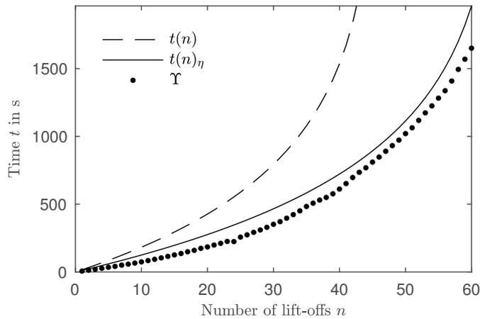
Fig. 7: Lift-off time with lift-off index. The theoretical prediction  $t(n)$  was found using the iterative model presented in section 2.3, as was the prediction including  $\eta$  (this was achieved by multiplying  $\Delta_c \rho$  by this factor). The measurement  $Y$  in this experiment was made with a small glass bottle and a Swiss 2-franc-coin.
