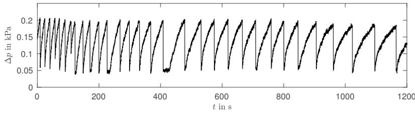
Fig. 3: Pressure difference with time (Optimal data). Particularly interesting is a data pattern precisely as suggested by the qualitative model: after having reached a critical pressure difference, the system pressure very rapidly drops to ambient pressure with the intervals between the lift-offs increasing in length.
