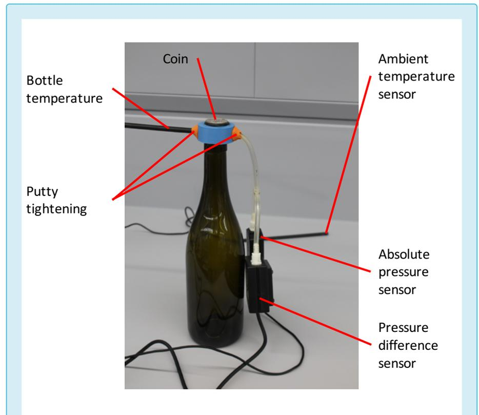
Fig. 2: Experimental setup. The tightening ring was latter omitted as it proofed to be redundant in later cap versions.
