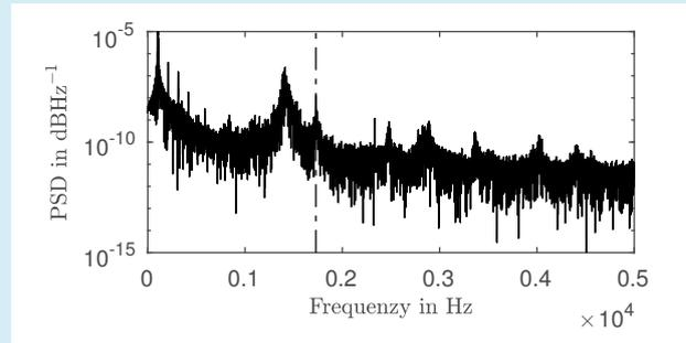
b) The frequency spectrum of the same bottle at a temperature of 263 K with enforced Helmholtz resonance. The lower peak indicated by the dashed line is at a frequency of  $f_7 = 1727$ Hz.
