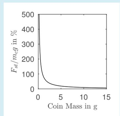
Fig. 10: Ratio between surface tension and coin weight with constant radius of roughly  $r = 1$  cm. For heavier coins, a bigger part of the force needed to lift it is its weight. It is therefore plausible that the pressure does not build up to the full pressure required by equation (2.10), but that the water tightening starts leaking before that due to the pressure, possibly explaining the large discrepancies observed in figure 6a and 6b.
