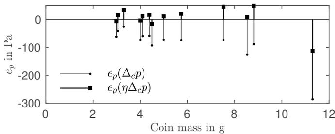
b) The residuals  $e_p$  of figure 6a that are given by a measured value  $Y$  and a predicted value  $P$  according to  $e_p = Y - P$ . There is no trend observable that would suggest the presence of a systematic deviation, but the residuals nicely show how the discrepancies in the model without the correcting factor  $\eta$  grow very large. The RMSE-value of the fitted line is 40.8.
