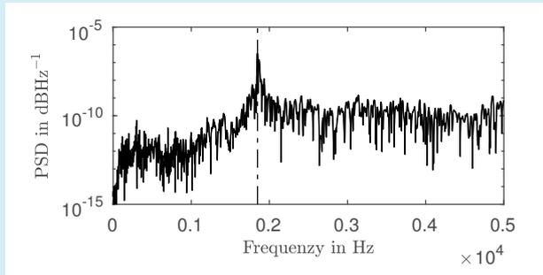
a) The frequency spectrum of a CHF 0.2- coin dropping onto the bottle (a larger spectrum of the same event is presented in the third spectrum from the top in figure 8) at a temperature of 293K. The black dashed line indicates the frequency with the highest spectral density at  $f_2 = 1848$  Hz.
