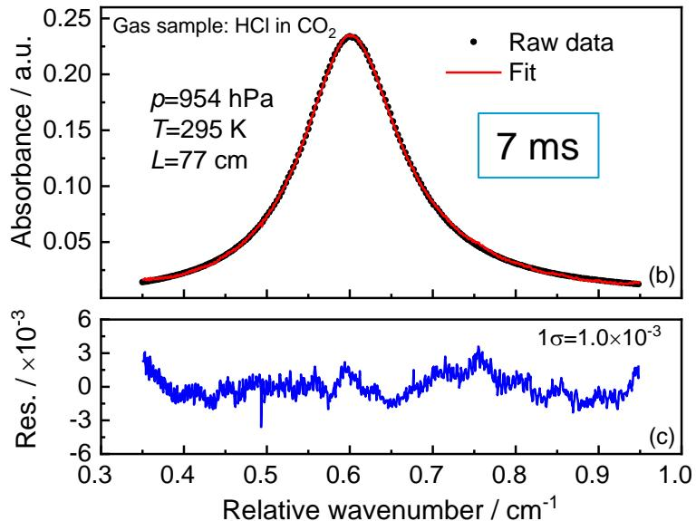
Instrument detection limit: 0.02 µmol/mol @ 1 s, 1 m
