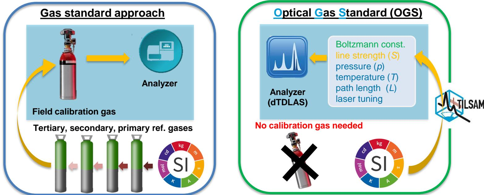
An **Optical Gas Standard** is a **laser spectrometer** that can provide amount of substance fractions (concentration) that are **directly traceable to the SI**
