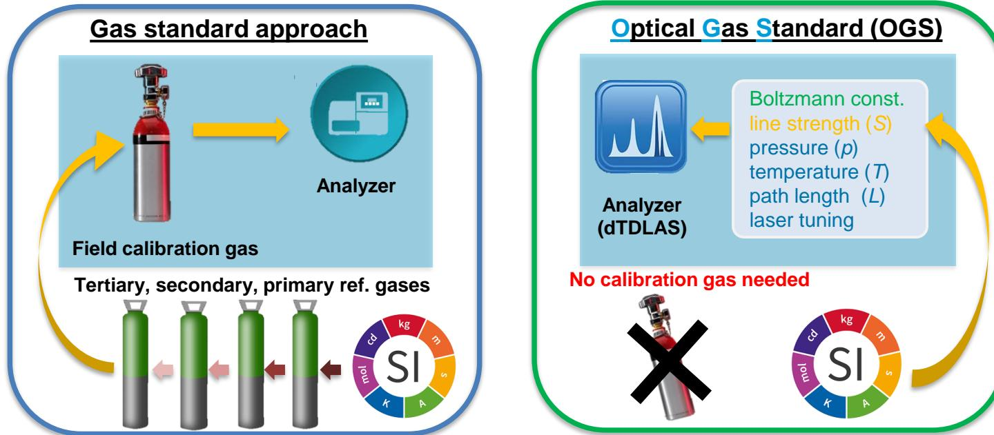
An **optical gas standard** is a **laser spectrometer** that can provide amount of substance fraction (concentration) results that are **directly traceable to the SI**
