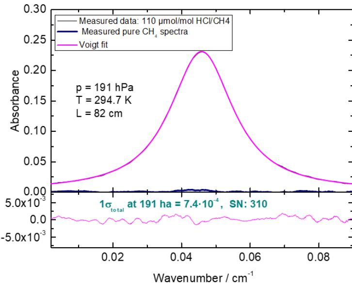
The detection limit of this HCl-OGS system is 29 nmol/mol at  $\Delta t = 54$  s
