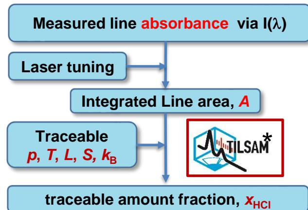
\*Traceable Infrared Laser-Spectrometric Amount fraction Measurement ([TILSAM](#)) > metrological description
