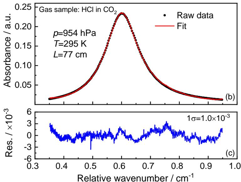
Instrument detection limit:  $0.02 \mu\text{mol/mol}$  @ 1 s, 1 m
