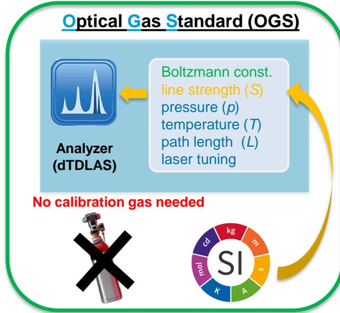
An **optical gas standard** is a **laser spectrometer** that can provide amount of **substance fraction (concentration)** results that are **directly traceable to the SI**
