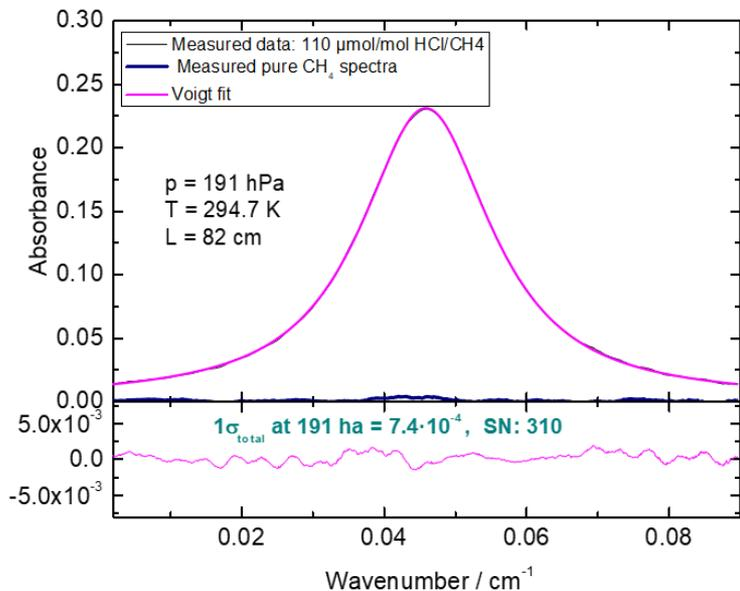
The detection limit of this HCl-OGS system is 29 nmol/mol at  $\Delta t = 54 \text{ s}$
