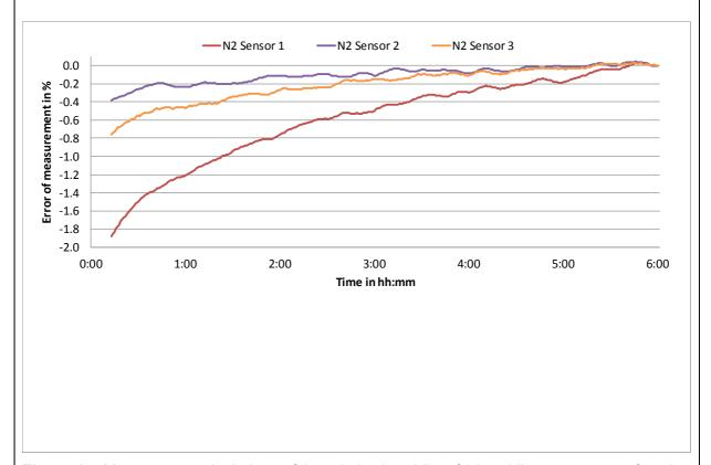
**Figure 17:** Measurement deviations of the relative humidity of 3 humidity sensors as a function of time at calibration point N2
