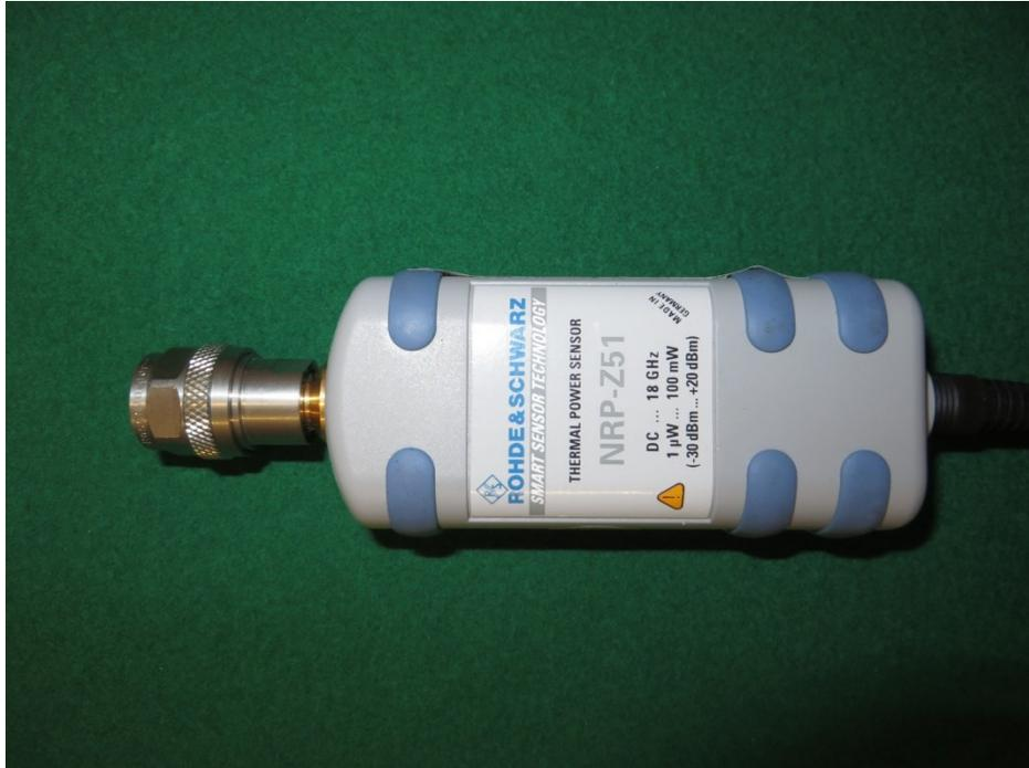
Figure 11.2.1: Measurement object *NRP-Z51* with serial number 104095
