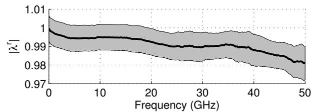
Fig. 3. Reflection coefficient  $\lambda^r$  of the used calibration standard.
