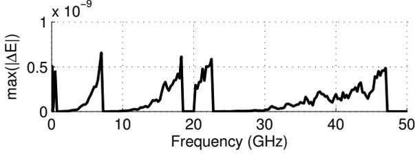
Fig. 4. Maximum difference of all error terms between the TRM calibration and the optimization calibration.
