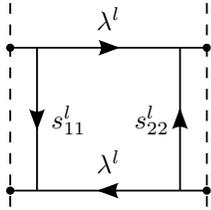
Fig. 2. Line standard with unknown transmission  $\lambda^l$ .
