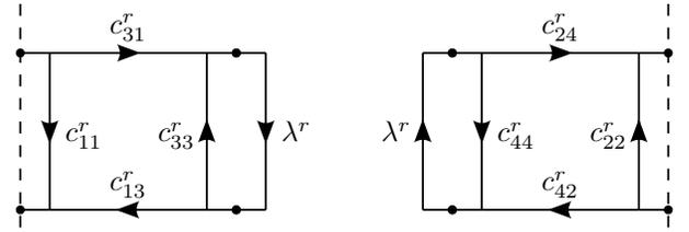
Fig. 5. Two two-ports,  $c$ , representing connector repeatability uncertainties, are cascaded to the two one-port standards with the same unknown reflection  $\lambda^r$ .
