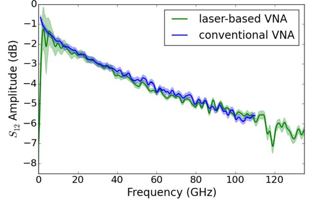
Fig. 2: Amplitude of  $\mathbf{S}_{12}$  of the DUT obtained from the time- and frequency-domain techniques (thick lines). The 95% confidence intervals are marked by the light semi-transparent colors.
