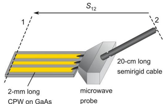
Fig. 1: Device under test and definition of scattering parameters.
