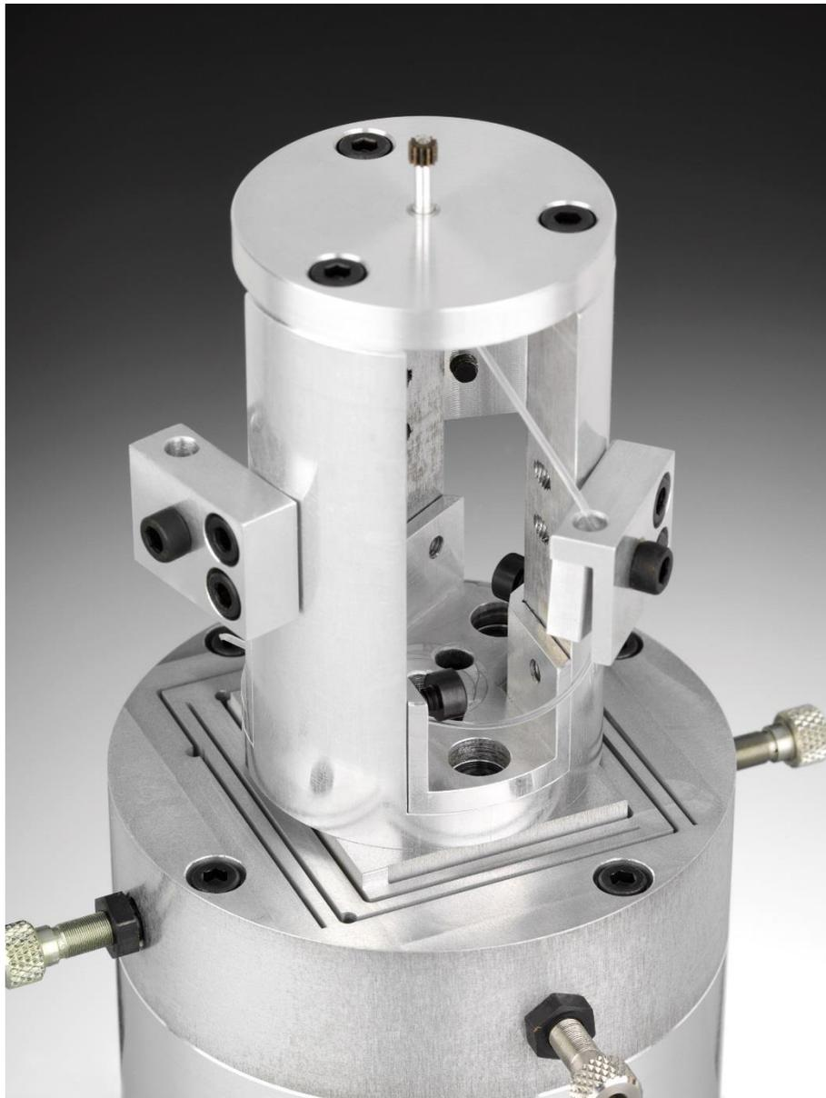
Figure 2: Upper part of the prototype featuring the compliant string clamp. The string material is fluorocarbon and the monofilament has a diameter of 0.9 mm
