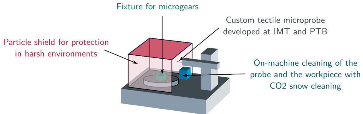
Figure 7: Integration of the compliant string clamp in a microenvironment that features a particle shield, cleaning capability and several sensors that monitor the direct measurement environment (vision system, temperature and humidity sensor, sensor for airborne particles)
