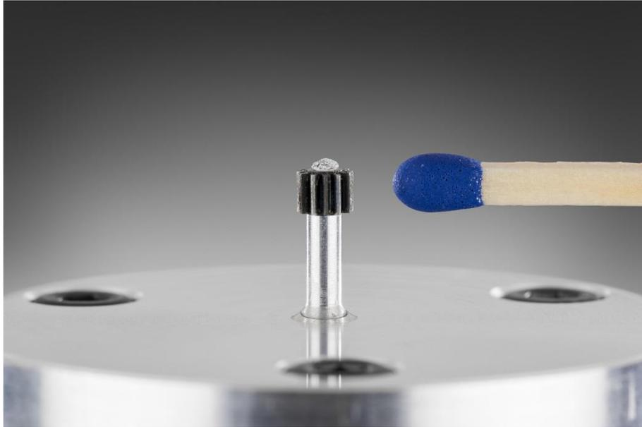
Figure 3: Close-up of the clamped microgear in comparison with a match head. All clamp components (tube and string) are low-cost, mass-produced goods
