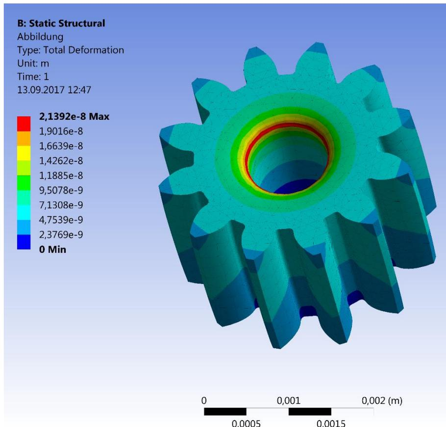
Figure 4: FEM simulation of the string clamp. Deformation and stress invoked by the fixation are comparable to collet clamping and fixation with a three-jaw chuck
