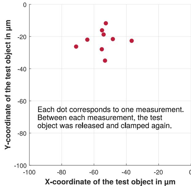
Figure 5: High repeatability after reclamping of the same workpiece, enabling automation of the measurement process since the residual eccentricity is compensated by software of the measuring machine
