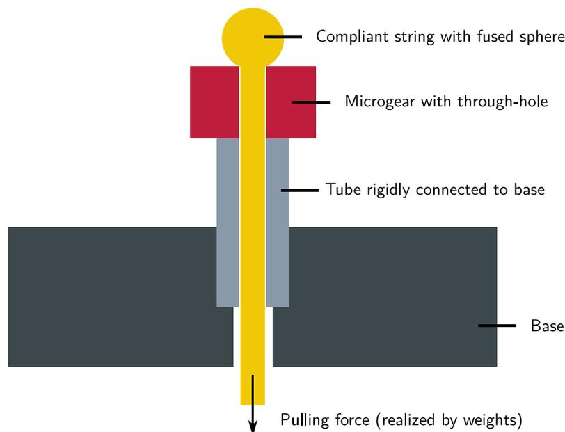
Figure 1: Schematic overview of the new microclamping principle for microgears. The string centers the microgear with respect to the tube. This method allows virtually every workpiece with through-hole diameters down to a few micrometers to be clamped. Threading of a workpiece may facilitate transport and handling
