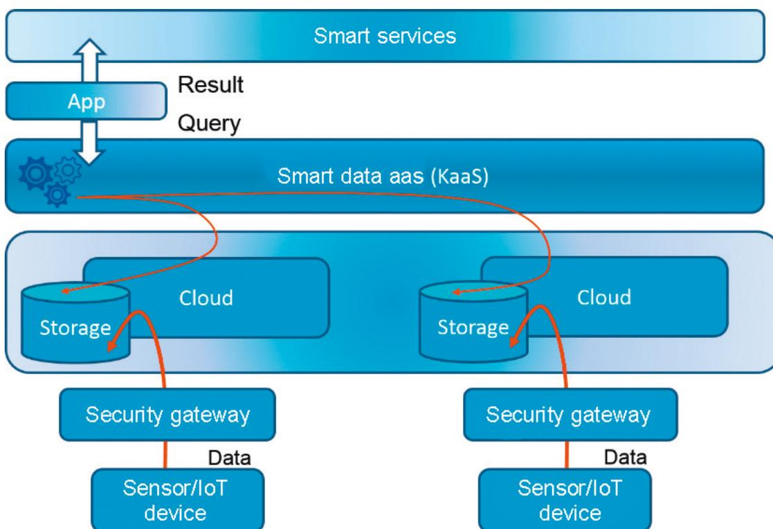
Figure 5: The basic technology stack of an IoT system. KaaS: knowledge as a service.
