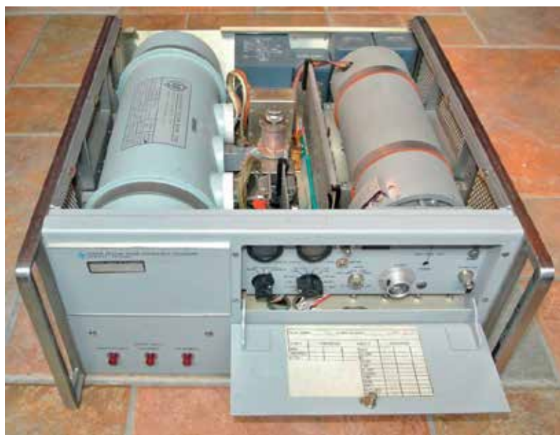
Figure 9: Hewlett-Packard 5060A cesium beam atomic clock with cover removed showing beam tube on left (courtesy of Tom Van Baak, leapsecond.com).
