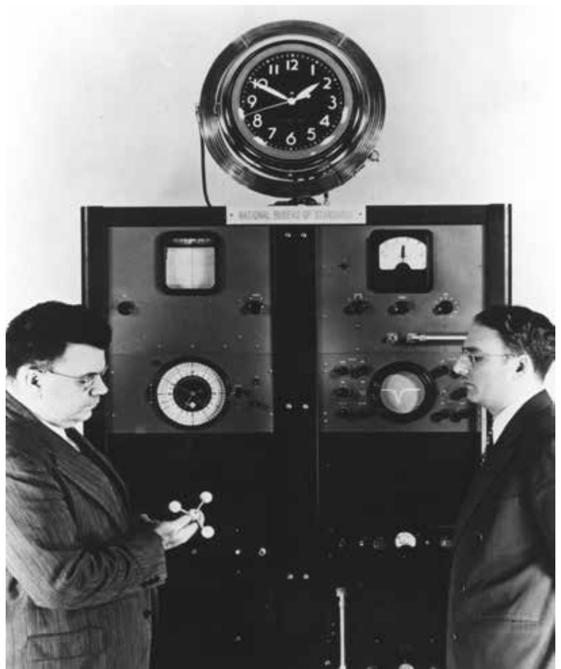
Figure 2: Dr. Harold Lyons (right), inventor of the ammonia absorption cell atomic clock, observes, while Dr. Edward U. Condon, the director of the National Bureau of Standards, examines a model of the ammonia molecule (1949). The clock atop the equipment racks was driven by a 50 Hz signal obtained by dividing the signal from a quartz oscillator that was locked to the ammonia absorption frequency. However, its primary function was to let the world know that the invention was indeed a clock.
