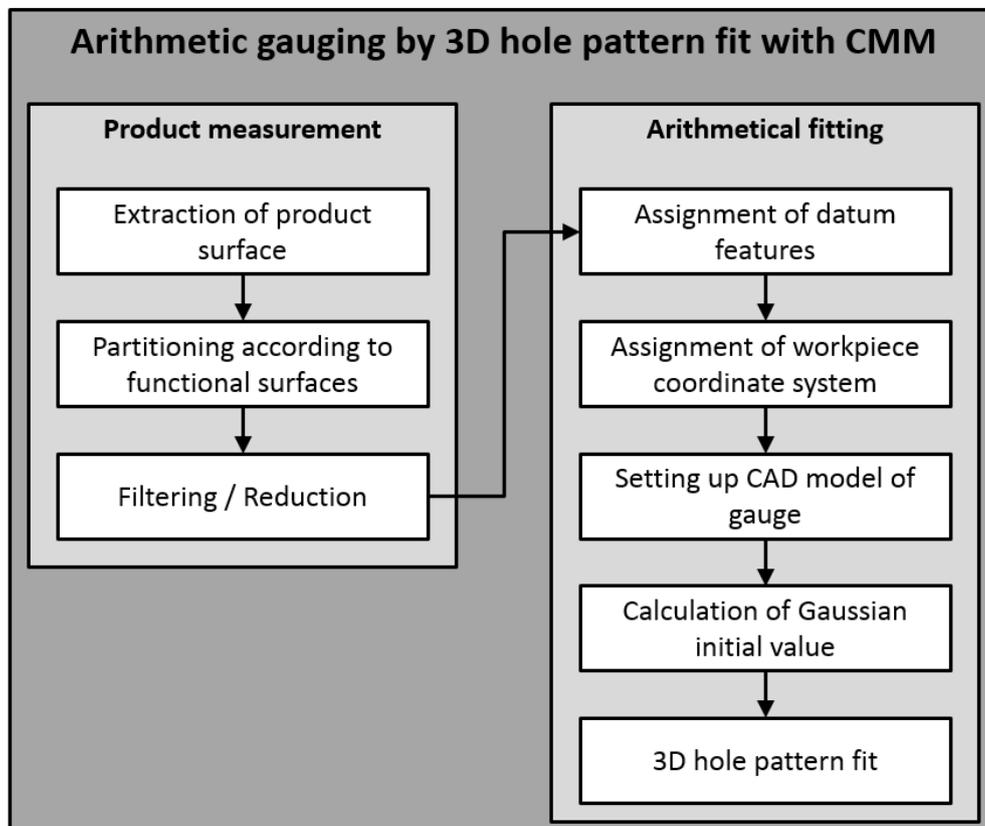
**Figure 3** Principal procedure of the arithmetic gauging by means of coordinate measurement machines.
