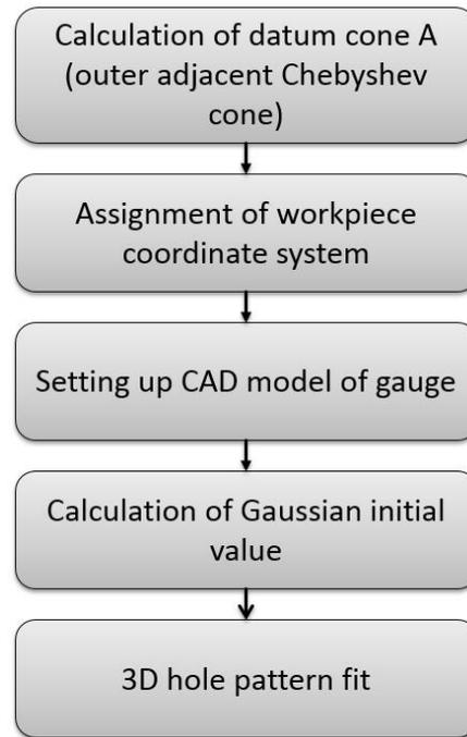
**Figure 19** Flowchart for 3D hole pattern fit for a conical disk.
