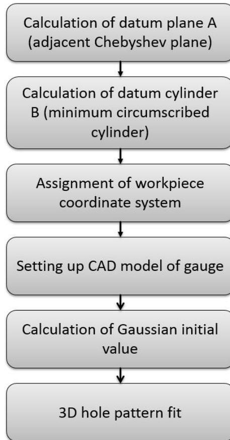
**Figure 10** Flowchart of the 3D hole pattern fit for the flange.
