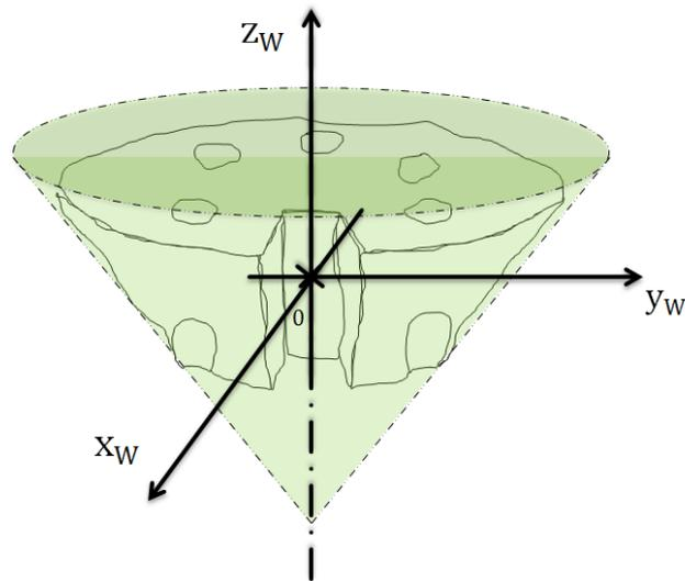
**Figure 20** Workpiece coordinate system for the conical disc
