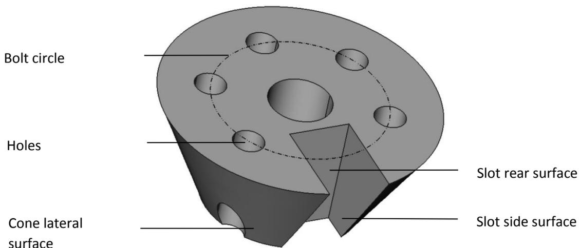
Figure 15 Example of a conical disc
