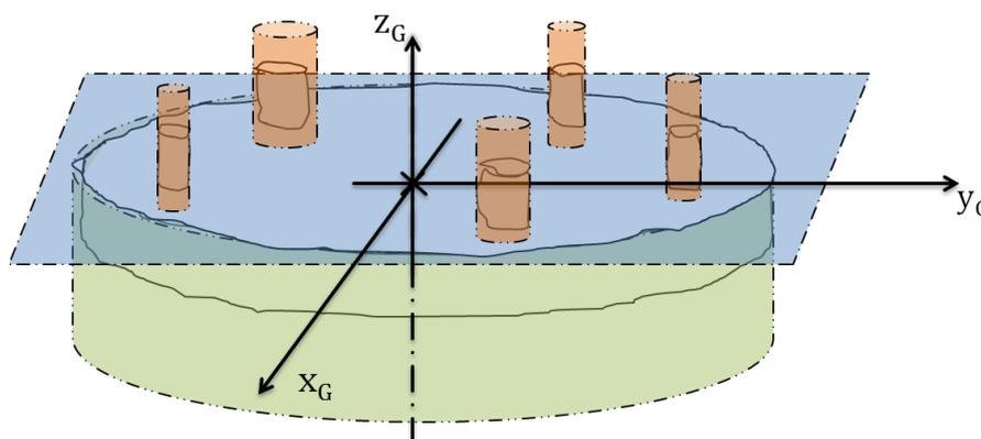
**Figure 14** Assignment of the virtual gauge to the counterpart.
