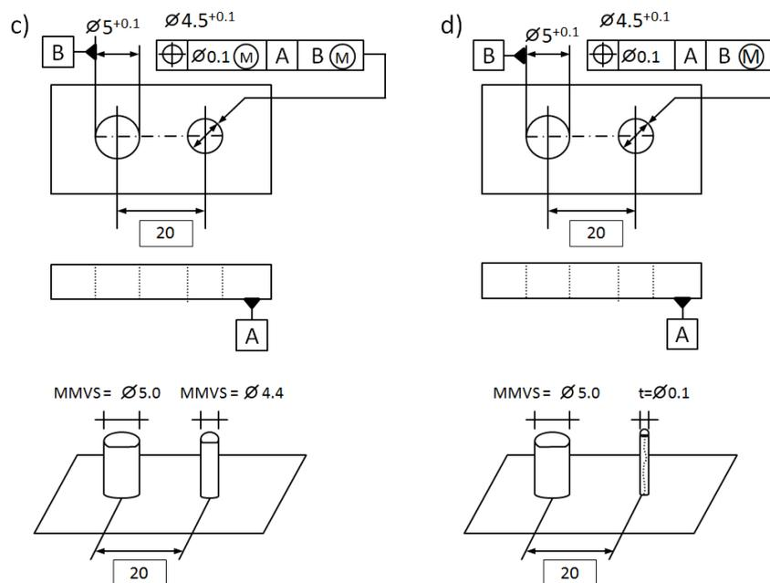
**Figure 2-2** Tolerances with datum features including drawing specifications  $\textcircled{M}$ .
