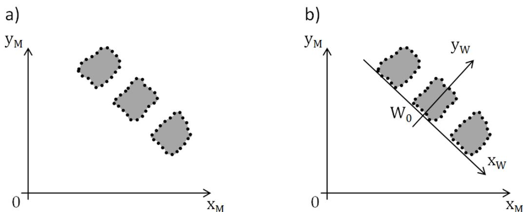
**Figure 4** Workpiece datum systems: a) extracted workpiece geometry in measuring machine coordinates, b) Alignment of the workpiece coordinate system at the lower edge of the extracted product.
