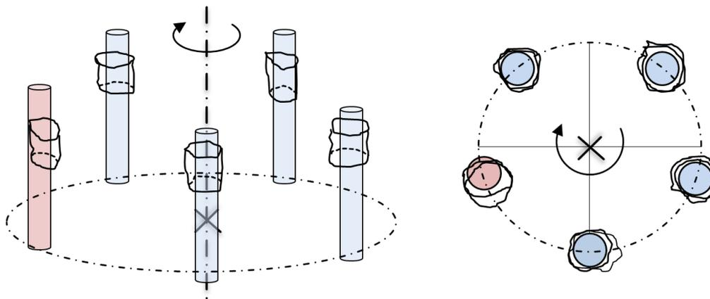
**Figure 9** 3D hole pattern fit for the flange (on the left: perspective view, on the right: top view); the gauge cylinder highlighted in red overlaps with the hole. By rotating all gauge cylinders around the datum axis, no position is found where all cylinders lie within the holes.
