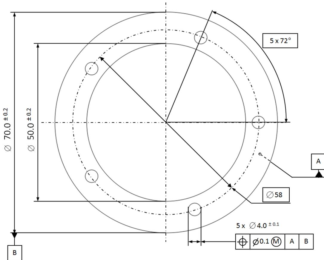
**Figure 7** ISO 1101 compliant inspection of the flange.
