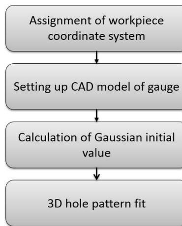
**Figure 24** Flowchart on the 3D hole pattern fit for the cube.
