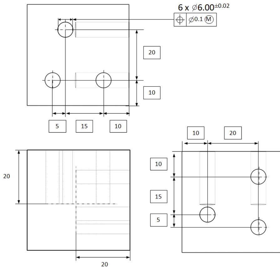
**Figure 23** ISO 1101 compliant inspection task for the cube.
