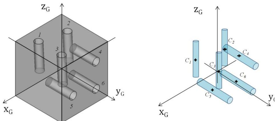
**Figure 25** Coordinate system and model of the virtual gauge for the cube.
