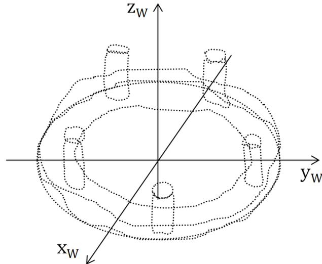
**Figure 11** Workpiece coordinate system and extracted geometry at the flange.
