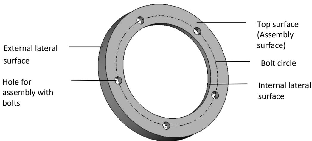
Figure 6 Application example of flange
