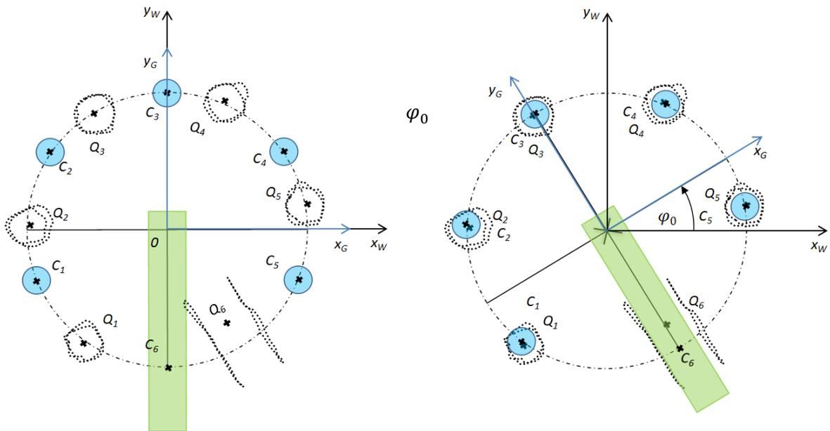
**Figure 21** Initial value of the conical disc fitting.
