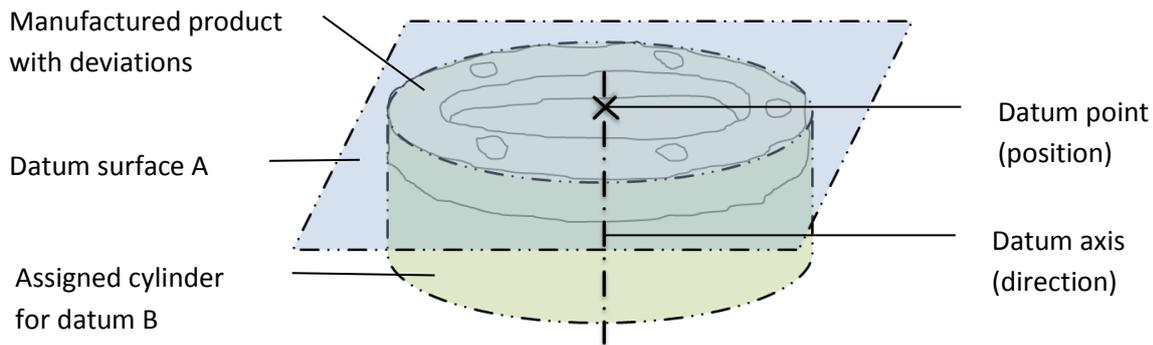
**Figure 8** Datum assignment at the manufactured flange.
