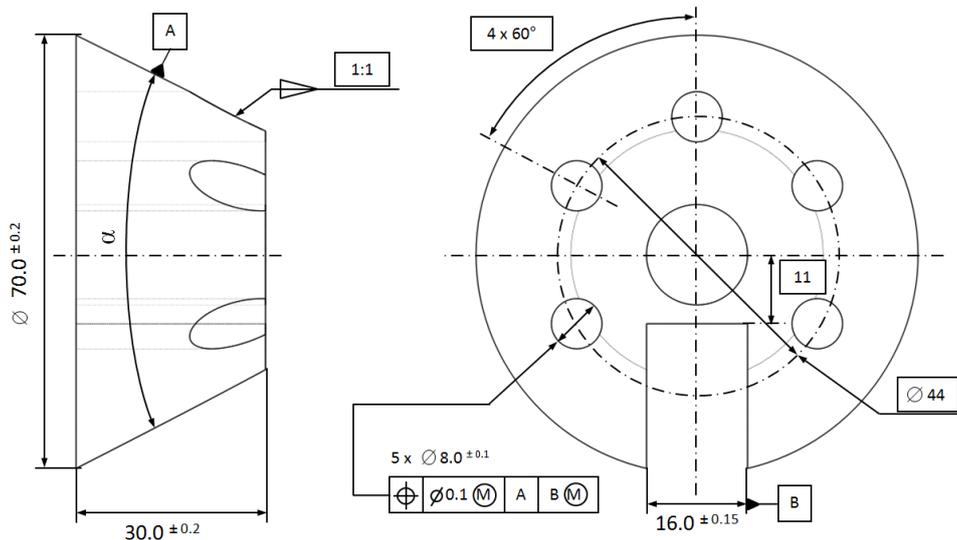
**Figure 16** Tolerancing for the conical disc (basis ISO 1101).
