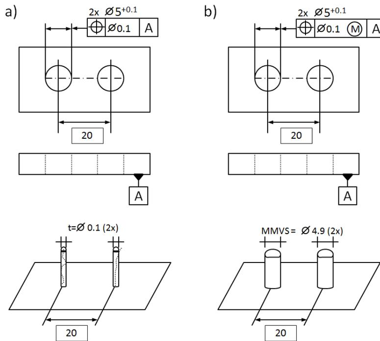
**Figure 2-1** Two examples for tolerancing a plate with two holes. The virtual inspection of the tolerances presupposes the 3D hole pattern fit in both cases (Tolerance principle ISO 8015).
