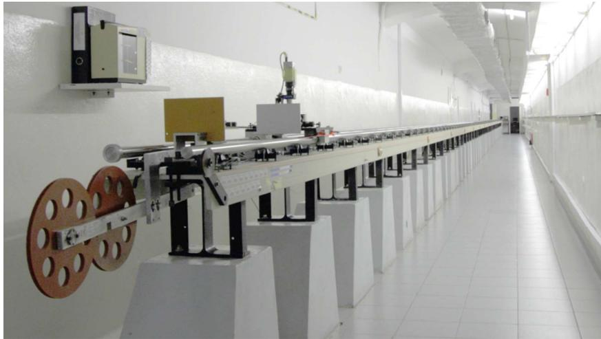
Figure 1: The 50 m interferometric comparator.
