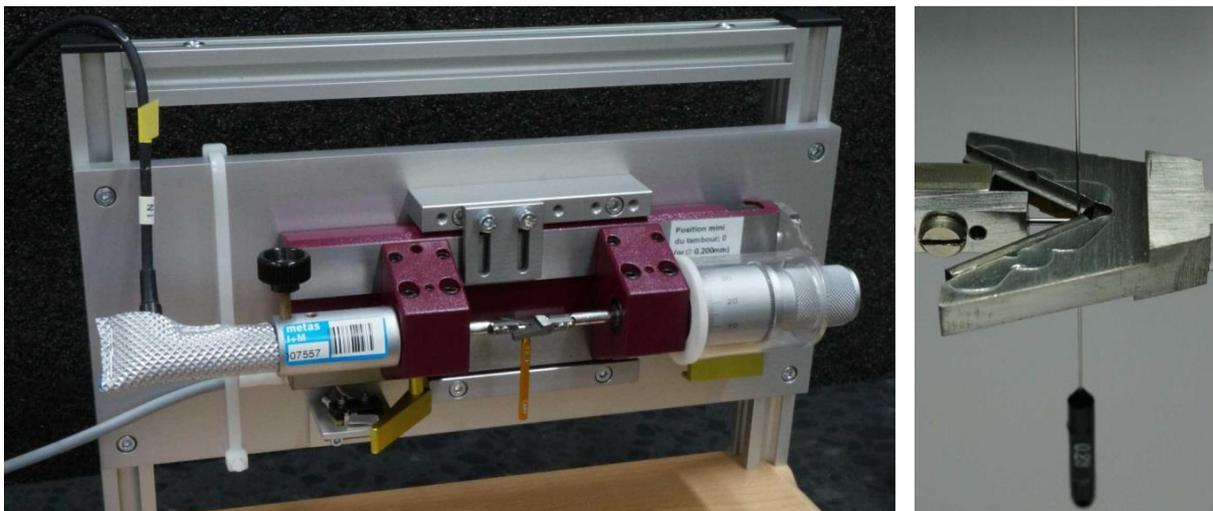
Figure 6: Three-point measuring instrument with a V-shaped anvil for the measurement of roundness deviation of pin gauges with diameter down to 0.2 mm.
