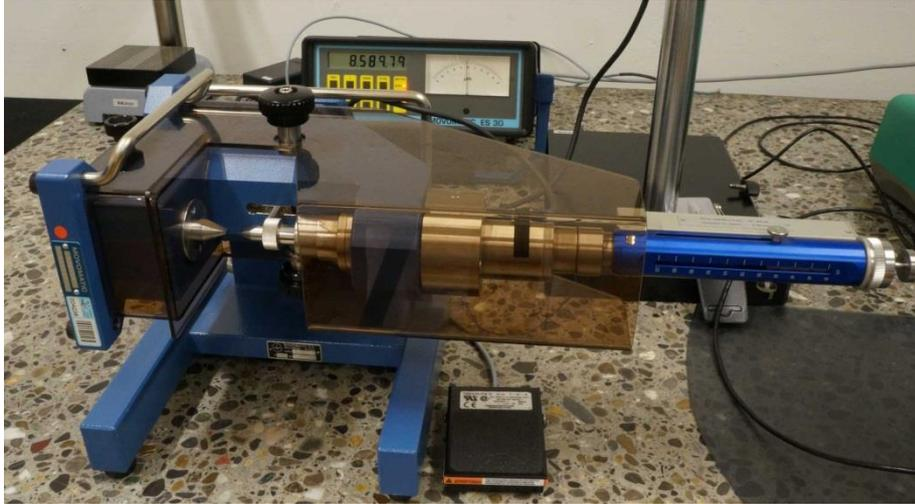
*Figure 3: Movotelit Abbe type comparator with an incremental length measuring system and flat anvils for pin gauge calibration.*
