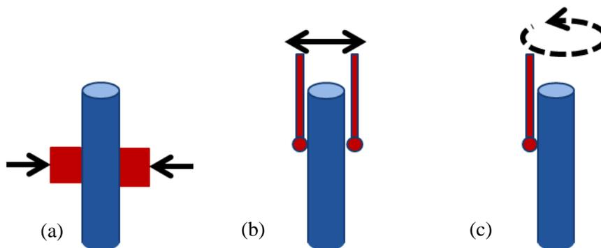
Figure 2: Three different tactile pin gauge calibration methods: (a) Length comparator with two flat probes, (b) 1D displacement comparator with spherical probe, (c) 2D or 3D measuring instrument with spherical probe.
