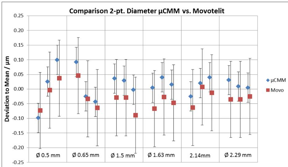
Figure 8: Comparison of diameter measurements between the Movotelit length comparator and the  $\mu$ CMM for six different pin gauges, at three different heights of each gauge. Error bars are expanded uncertainties with  $k = 2$ .
