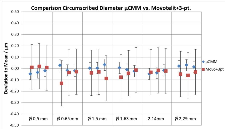
Figure 10: Comparison of circumscribed diameter values, measured by the  $\mu\text{CMM}$  and determined as the sum of average two-point diameters measured on the Movotelit and three-point centerless roundness values, at three different heights of each gauge. Error bars are expanded uncertainties with  $k = 2$ .
