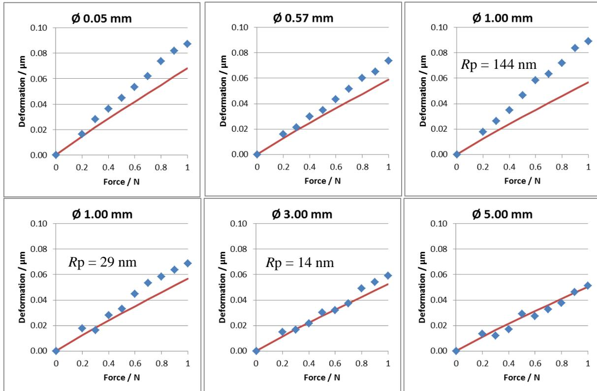
Figure 4: Elastic compression measurements for six pin gauges from steel with diameters between 0.05 mm and 5 mm on a length comparator with flat parallel tungsten carbide anvils of 1 mm width.
