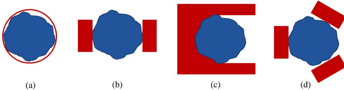
*Figure 1: Four different measurands for different applications of pin gauges: (a) Circumscribed diameter for limit gauging, (b) two-point diameter for the use as a setting standard for mechanical comparators, (c) two-point diameter for the use as a setting standard for optical comparators (laser scanners), or (d), three-point diameter for wires for screw gauge calibration.*
