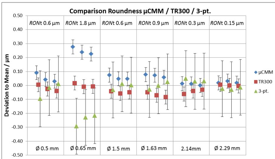
Figure 9: Comparison of roundness measurements between the three-point centerless roundness instrument, the TR300 form tester and the  $\mu$ CMM for six different pin gauges, at three different heights of each gauge. Error bars are expanded uncertainties with  $k = 2$ .
