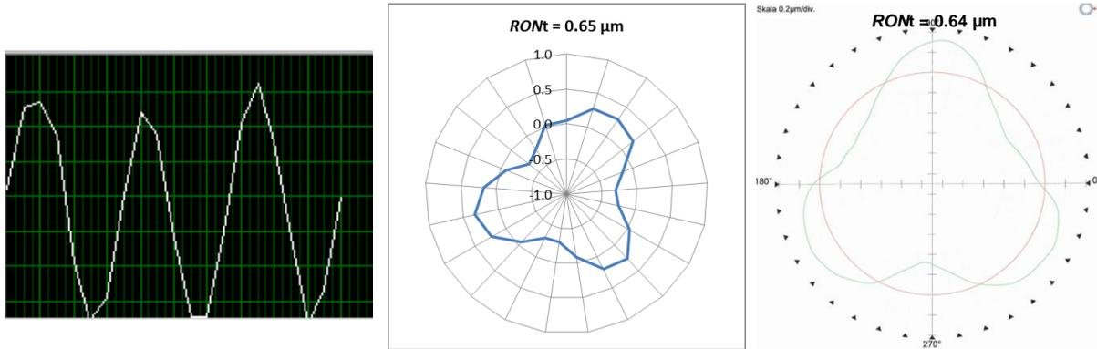
*Figure 7: Three-point diameter variation (left) of a 1.5 mm pin gauge as recorded by the centerless roundness measuring instrument, polar representation of this measurement (middle) and roundness measurement with a rotating spindle instrument (right) for comparison.*
