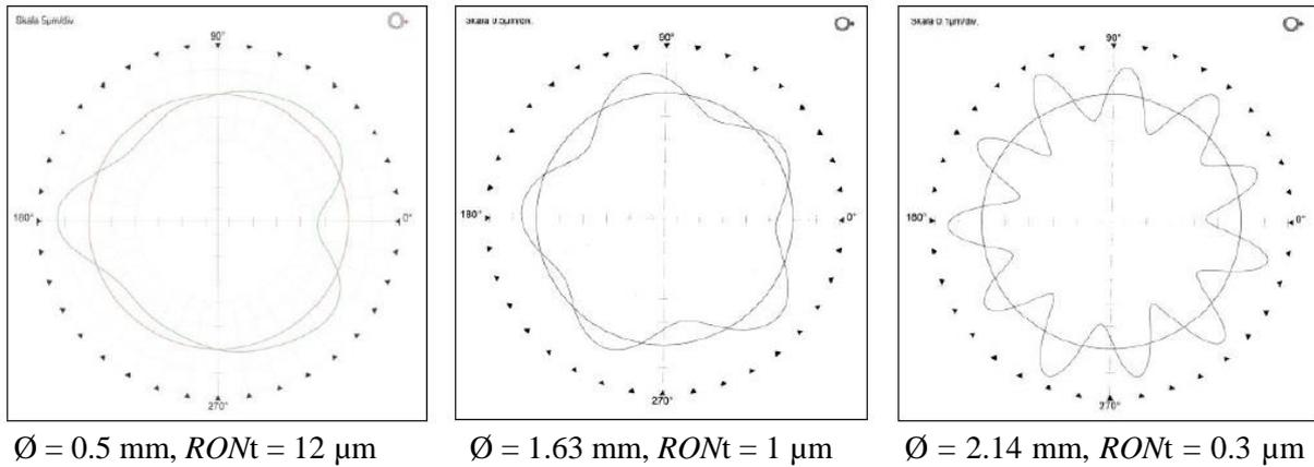
Figure 5: Examples of centerless machined pin gauges with large constant diameter form deviations with 3, 5 or 11 lobes. The roundness measurements were made with a Talyrond 300 form tester.
