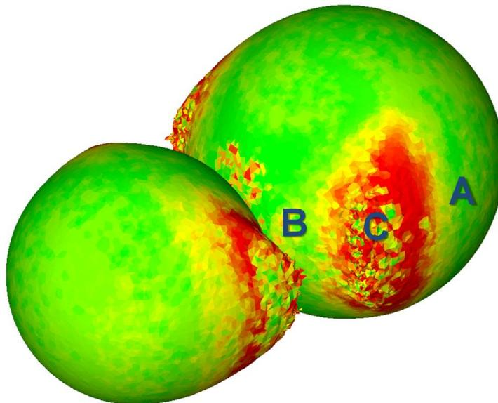
Figure 4: Basic principle of the determination of the LQV portrayed on a CT scan of two touching steel spheres (diameters 5 and 6 mm). The LQV is assessed by evaluating the sharpness and symmetry of the transition from low to high grey values on a line perpendicular to the surface. Areas with incorrect surface determination (C) are reliably identified as low-quality surface points and marked as red. Surface points with a high LQV (A) are represented as green.
