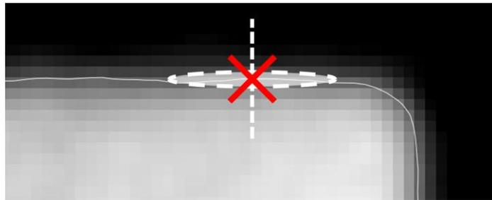
*Figure 3: Zoom of a cross section of the volume data. The red 'x' marks an extracted surface point. The grey values are extracted from a line perpendicular to the surface and an area along the surface, marked in white.*
