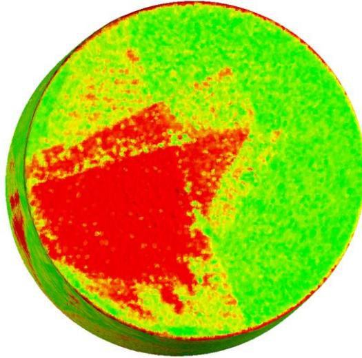
*Figure 6: Colour-coded representation of the LQV for a CT-scan of a cylinder (aluminium; height 12 mm, diameter 18 mm) with several layers of adhesive tape attached. The LQV is assessed by evaluating the homogeneity of the grey values along the surface and the sharpness of the transition from low to high grey values on a line perpendicular to the surface*
