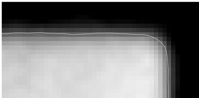
*Figure 1: Zoom of a cross section of the volume data, the grey line represents the extracted surface. The edge is rounded off in the volume dataset, resulting in the same effect in the surface dataset.*
