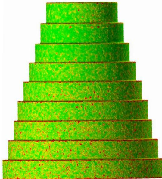
*Figure 5: Colour-coded representation of the LQV for a CT-scan of a hollow step cylinder (acrylic glass; height 45 mm, maximum diameter 42 mm). The LQV is assessed by evaluating the homogeneity of the grey values along the surface. Low quality surface points are identified at edges and for longer penetration lengths.*
