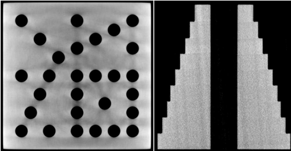
*Figure 2: Cross sections of an hole plate (aluminium; left) and step cylinder (acrylic glass; right). Cupping and streak artefacts are induced by beam hardening. Due to longer penetration lengths for the lower steps of the cylinder, the level of noise is increased in this area.*
