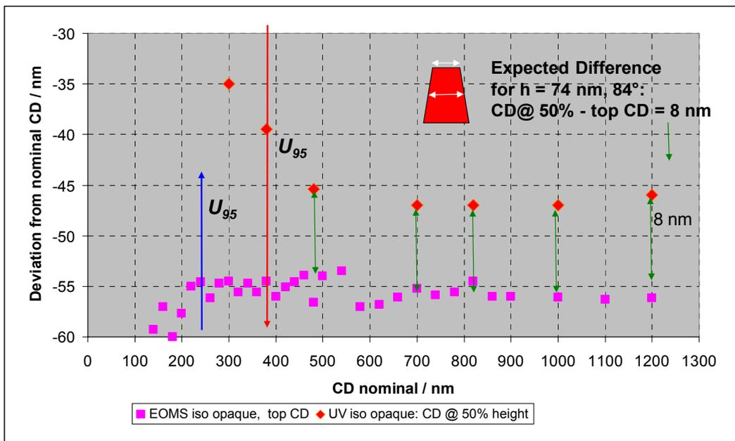
Figure 11: Results of a linewidth comparison between the UV-Linewidth-Microscope and the EOMS of isolated opaque chromium lines of a photo mask.
