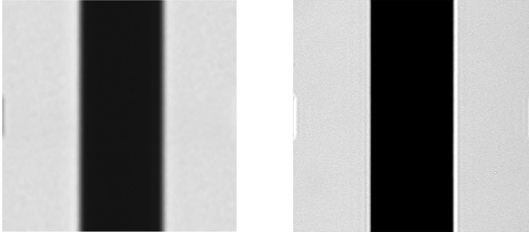
Figure 4: Images of a 10  $\mu\text{m}$  wide line taken by the same microscope using objectives with a numerical aperture of 0.3 (left) and 0.75 (right). The microscope operates in transmission mode.
