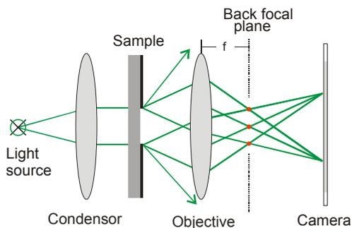
Figure 1: Image formation of an optical microscope
