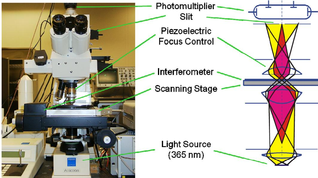
Figure 10: Line width calibration microscope
