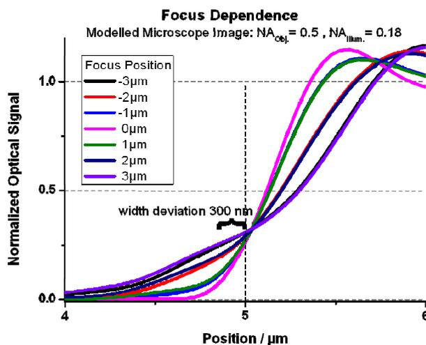
Figure 7: Defocus influence on the course of the edge profile of a 10  $\mu\text{m}$  wide line.
