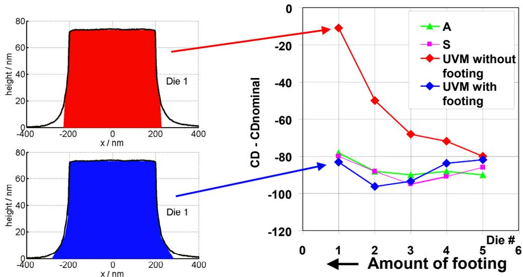
Figure 9: Influence of footing. Top: graphical description of the phenomenon in the simulation of the microscopic optical image. The black curves (envelopes) show the line cross sections measured by an AFM. Bottom: Change of the line width as function of the nominal linewidth if the footing is considered in the simulation and not (red and blue curves). For a comparison the AFM (green curve, A) and SEM (magenta curve, S) CD measurements are shown as well.
