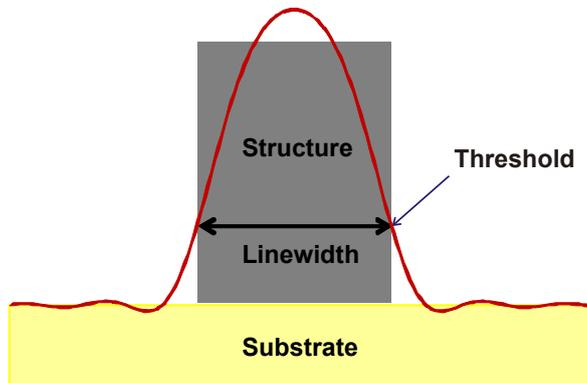
*Figure 2: Profile of a high reflecting line structure on a low reflecting substrate obtained by a reflection type microscope, the line edge is assumed to have ideally sharp edges, i. e. edges with an edge slope of  $90^\circ$*
