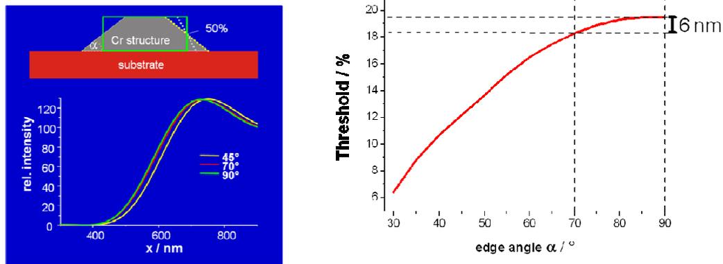
Figure 8: Influence of the line structure's edge angle. Left: Principle of the simulation and resulting profiles of the right edge for different edge angles. Right: Change of the threshold. The simulations are performed for a 1  $\mu\text{m}$  wide line (width constant at 50% of the height) and the linewidth calibration microscope described in detail below.
