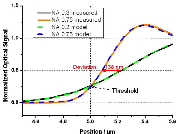
Figure 5: Simulated and image profiles taken from the images in figure 4 of the right edges.
