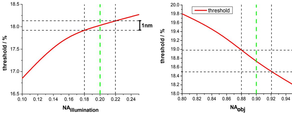
Figure 6: Influence of the numerical aperture of the microscope illumination and objective on the threshold for a 1  $\mu\text{m}$  wide line.
