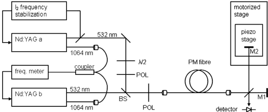
Figure 3: Simplified experimental setup of the interferometer
