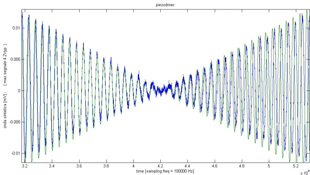
Figure 5: Typical interferogram at the minimum together with the fitting function (2)
